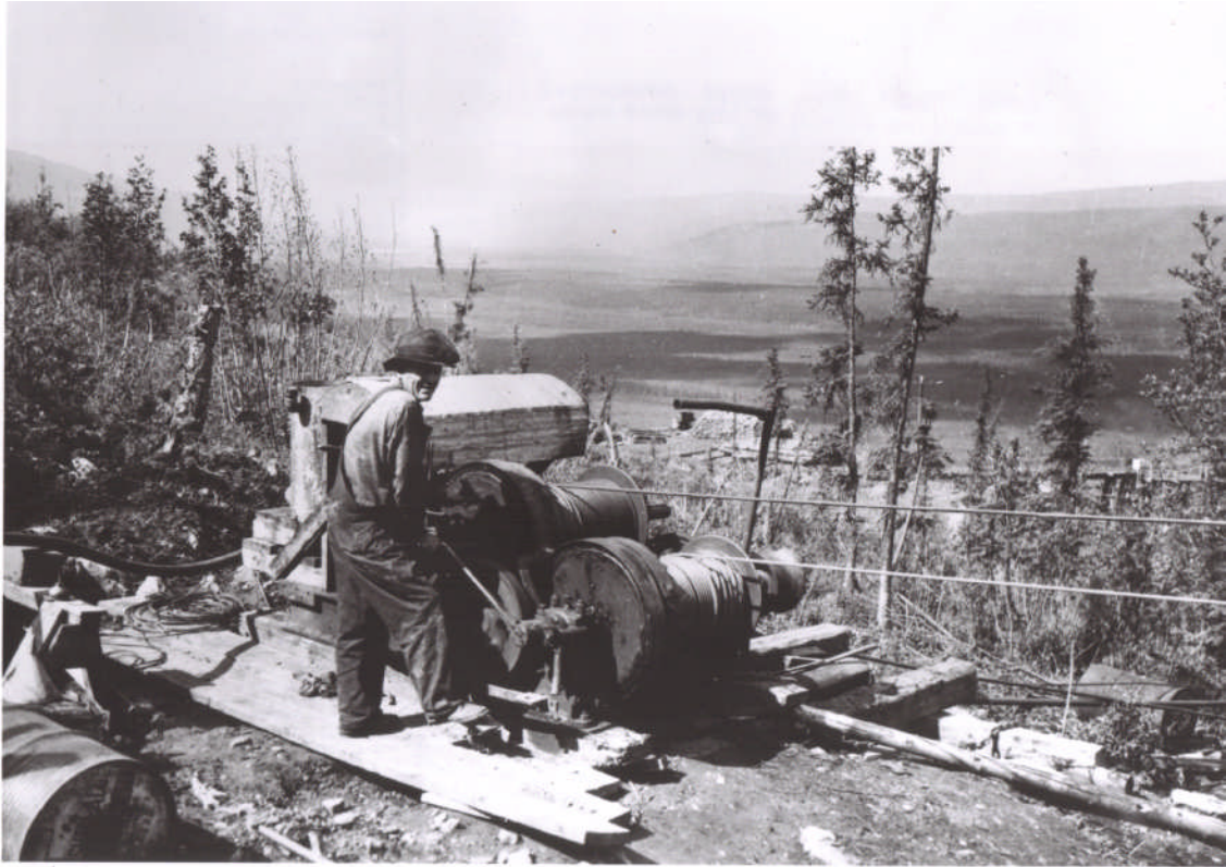
6998 - late 1930's Bill Boyle operating a dragline winch at the Elsa Mine
