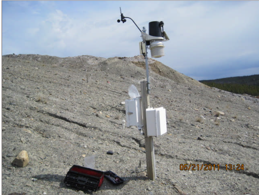
Photo 5: Davis Instruments Pro Vantage Weather Station located in CT#1.
