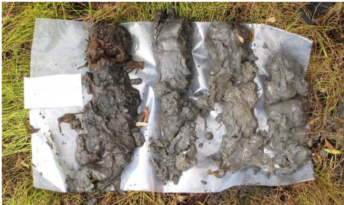
Photo 2. Sediment cores from a vegetated site up-gradient of Pond #1, showing tailings slimes and local sand within the lower intervals (the 3 right-most cores). Each core represents 15-20cm of sample depth.
