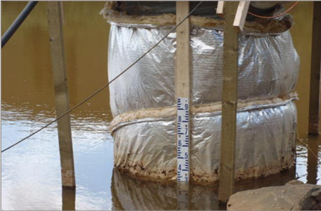
Photo 5: Re-installed Staff Gauge in the Seepage Pond. Installed July 18, 2012
