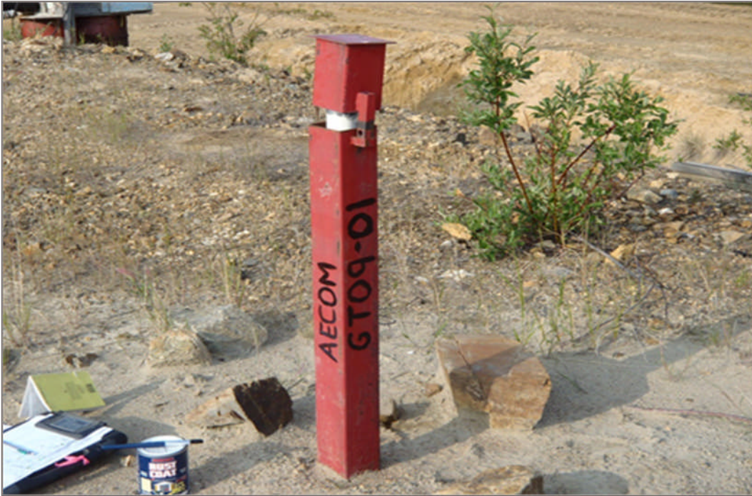
Photo 1: Example of a labelled borehole casing (July 18, 2012)
