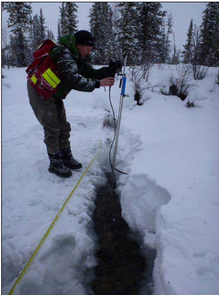
Photo 3. Winter velocity measurements using the Sontek FlowTracker meter on Victoria Creek.
