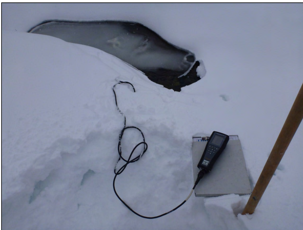
Photo 2. Salt dilution gauging with the YSI ProPlus Multi-Meter during the winter at Mount Nansen.
