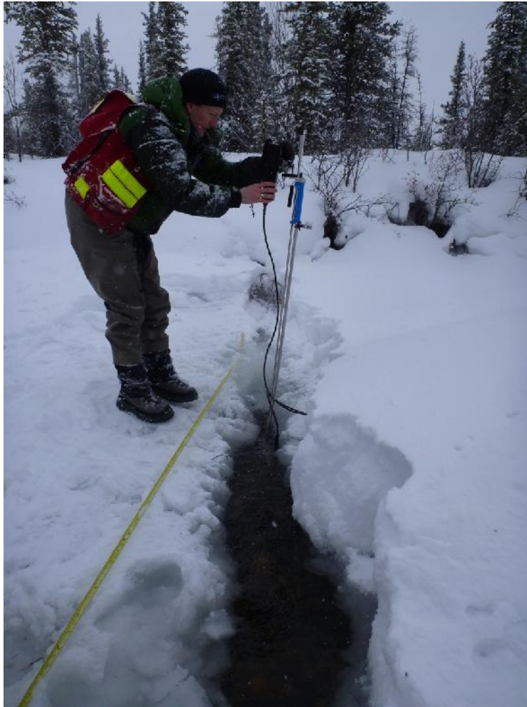
Figure 7. Winter velocity measurements using a current meter on Victoria Creek.
