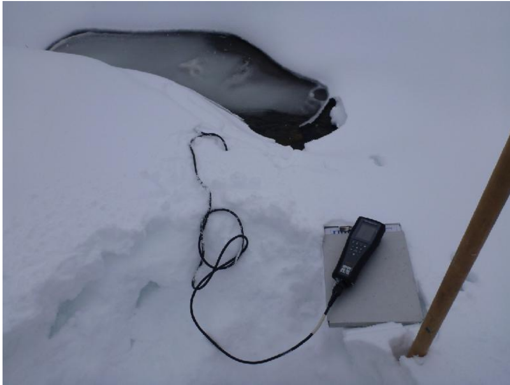
Figure 5. Salt tracer conductivity meter set-up. Salt input site was 90 m upstream of the conductivity meter.
