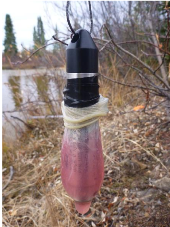
Figure 8. A winterized HOBO U20-001-04 water level logger.
