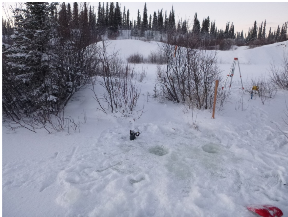
Photo 5. H-VC-R Thick overflow ice resulting in 88 cm of ice at the well site December 16, 2013.
