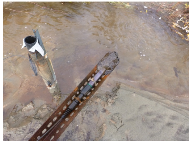
Photo 8. H-DC-M WP – logger showing sediment accumulation in stilling well.
