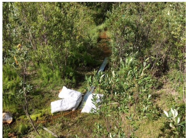
Photo 2. H-DC-DX+105 – looking downstream at metal trough installed for volumetric measurements.
