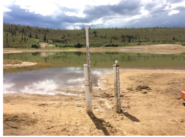
Photo 10. H-TP – overview of tailings pond showing dry staff gauges.
