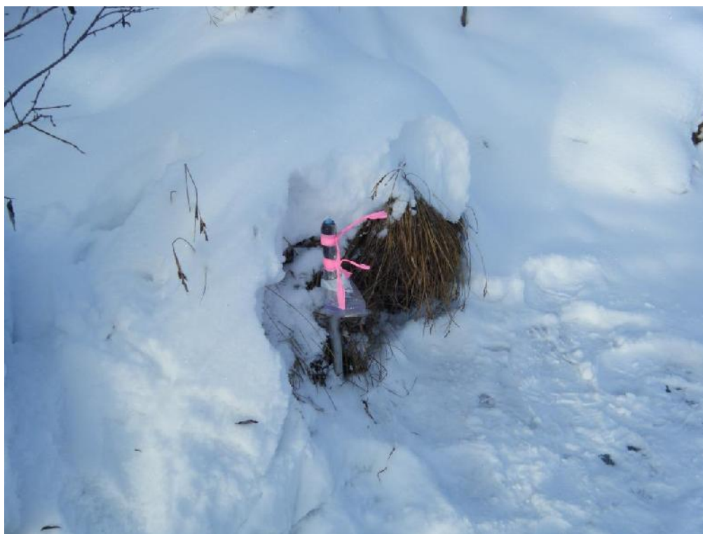
Photo 1. Piezometer CH13-107-PZ001 on right downstream bank, November 13, 2013.
