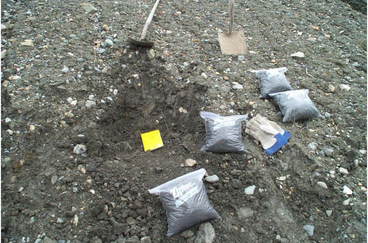
Photo 1: SRK-03-C01, till sample from the Vangorda waste rock pile cover. The sample excluded material that exceeded 50 mm (2'') in size
