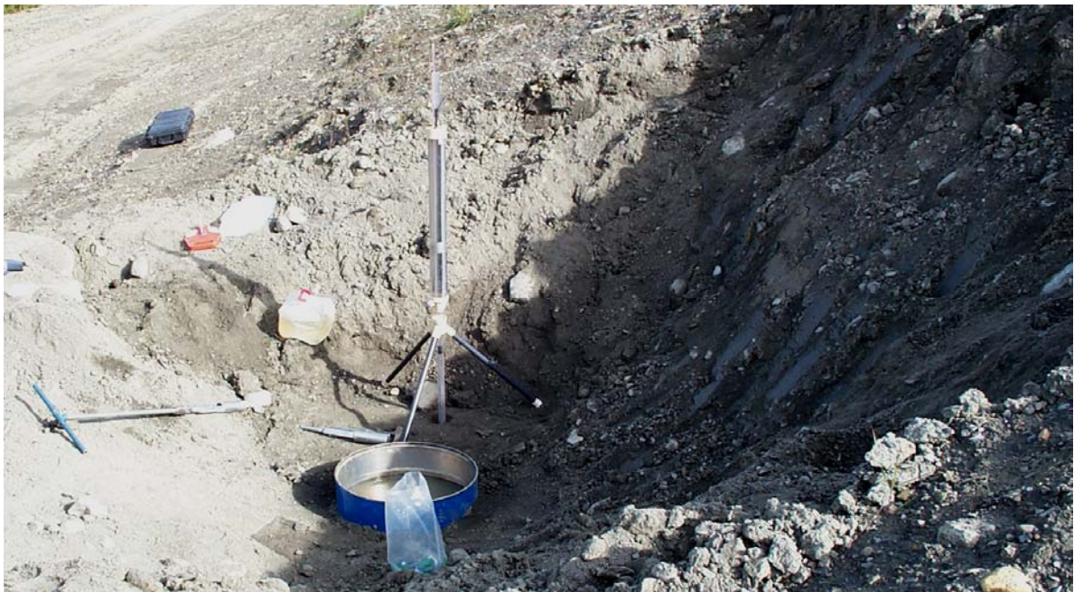
Photo 15: Test site showing a ring infiltrometer and Guelph permeameter.
