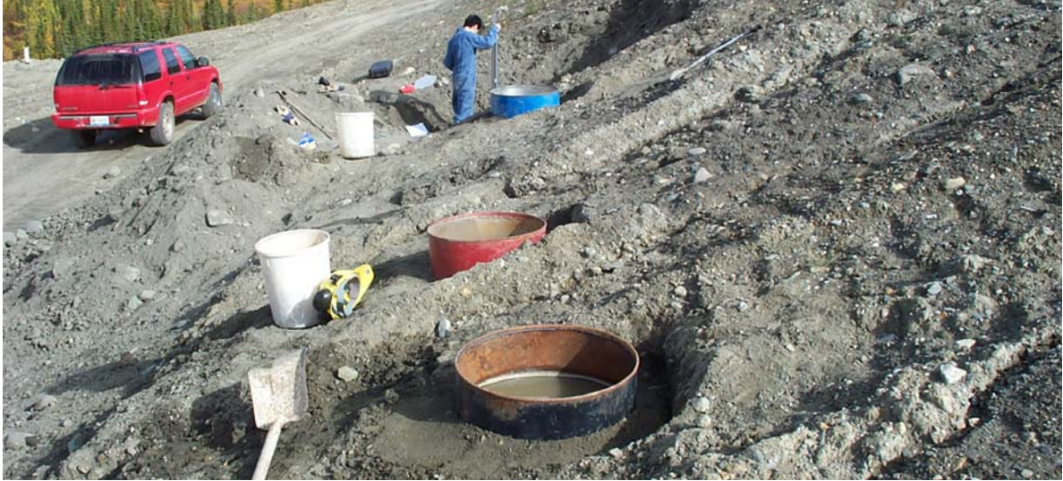
Photo 14: Sloped test site showing 3 ring infiltrometers being used for testing.
