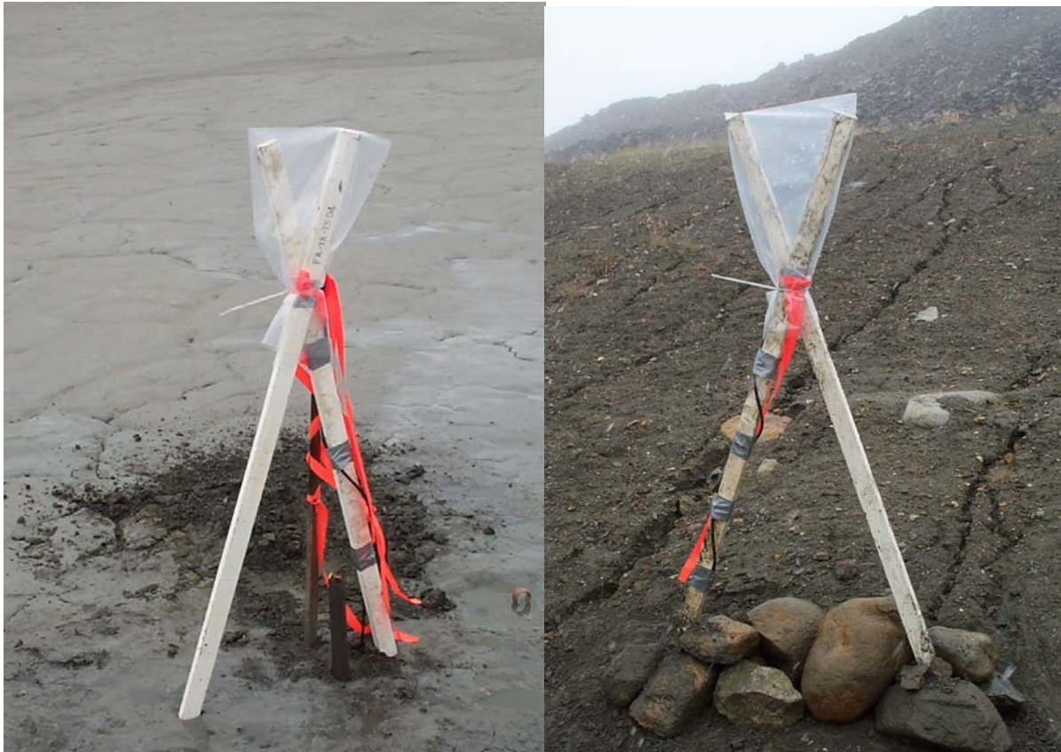
Photo 13: Examples of the thermistor installations on (1) Rose Creek tailings and (2) Vangorda waste rock pile starter dyke till.
