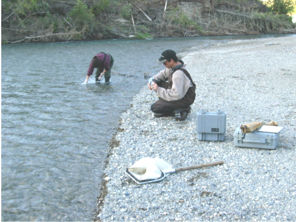
Plate 1. Collection of water samples for laboratory analysis and recording in situ measurements.
