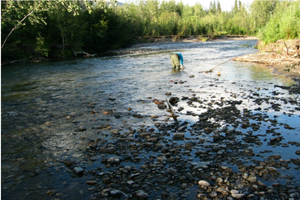
Plate 7. Benthic invertebrate sample collection at Site A2 to have tissues analysed for metals.
