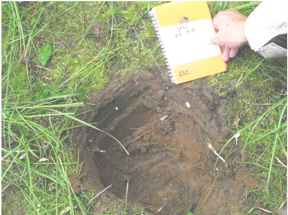
Plate 6 Soil sampling at test pit 5 of transect across the stream at Site A4 to have analyzed for metals and pH.
