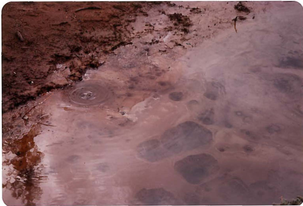
Seepage boils in abandoned meander of Rose Creek. Note active sand boil and craters from previous activity. Such boils are not a present concern.
