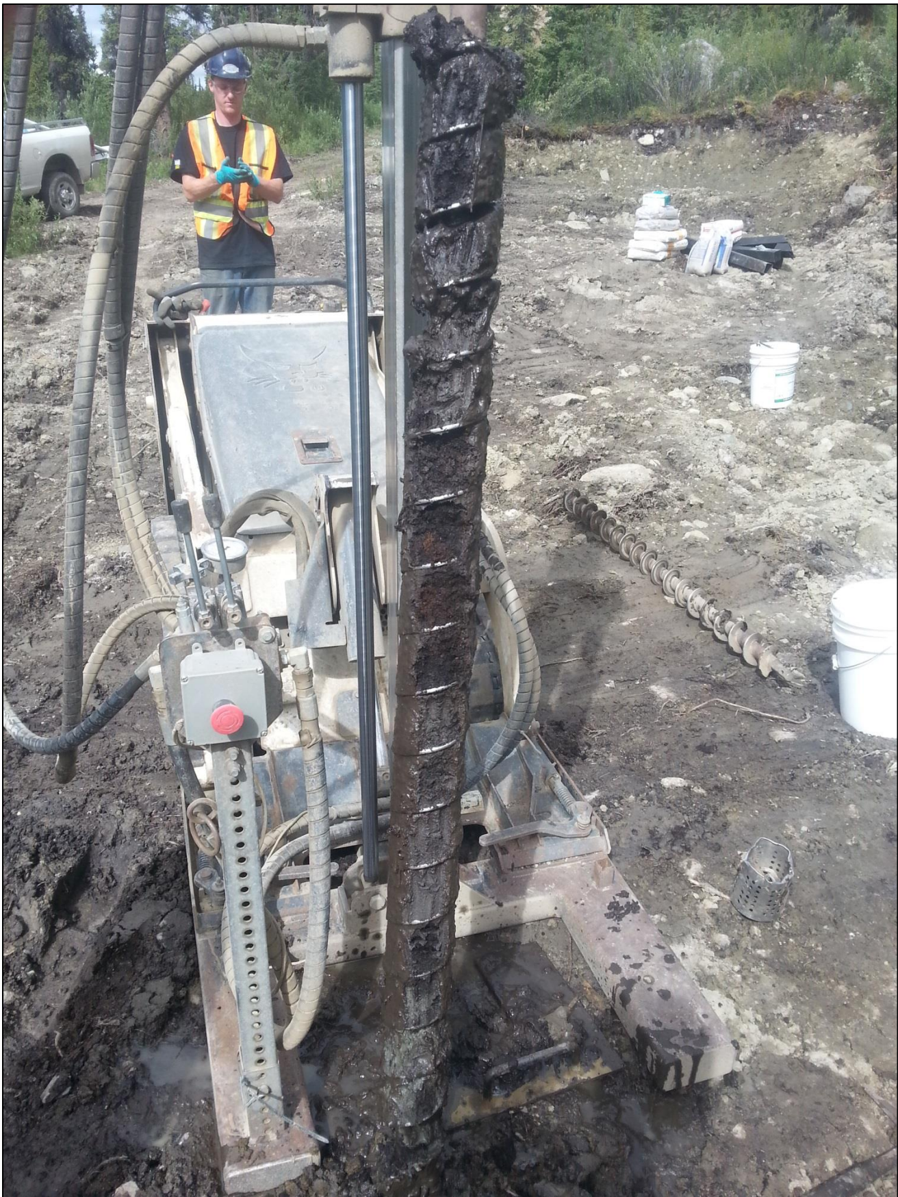
Photo A3: Sediment retrieved on auger flyte at MW14-08 (5-10 ft depth). The auger is screwed into the ground and then lifted straight out of the borehole, causing the sediment to stay in the grooves. The borehole is left unsupported and thus solid stem augers are only suitable in cohesive soils.
