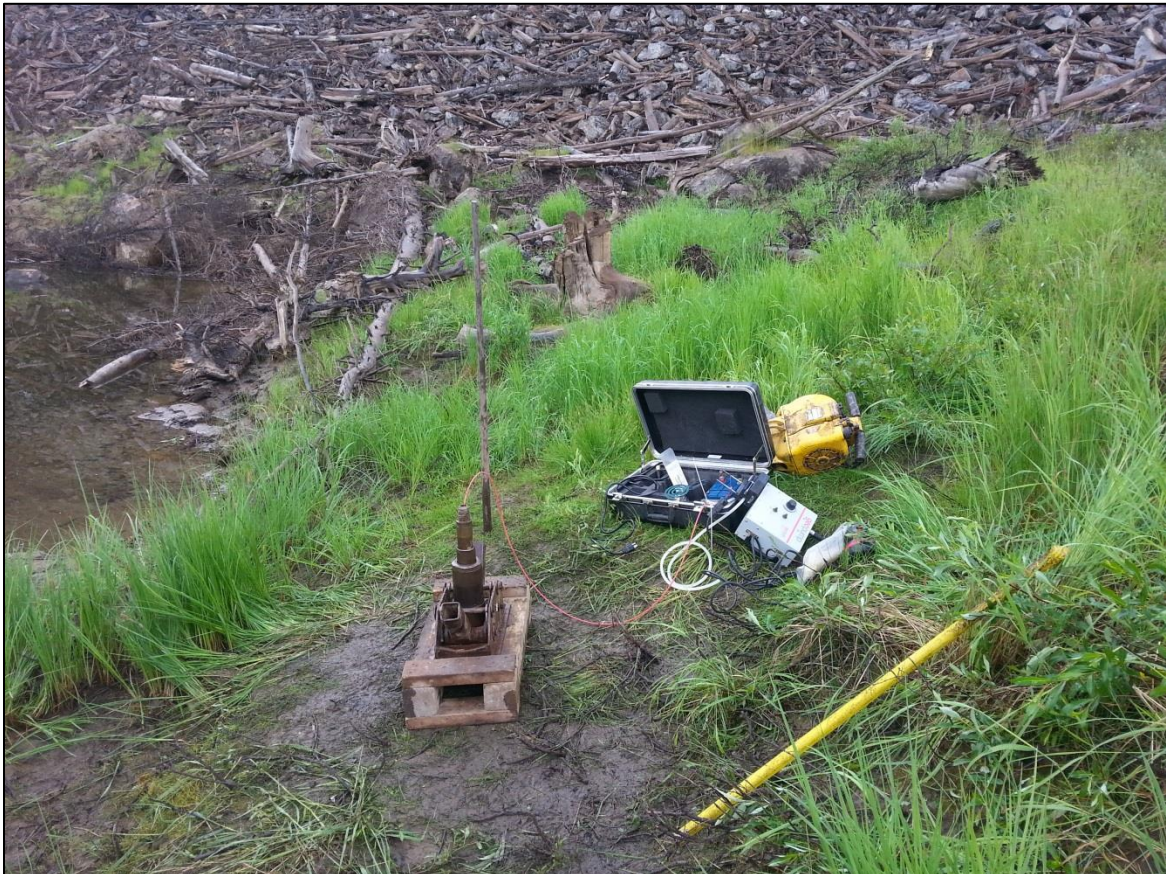
Photo A7: Using a peristaltic pump connected to the Waterloo profiler, a water sample is obtained from the sand aquifer at MW14-14. This was the water sample that contained 21 mg/L dissolved zinc.
