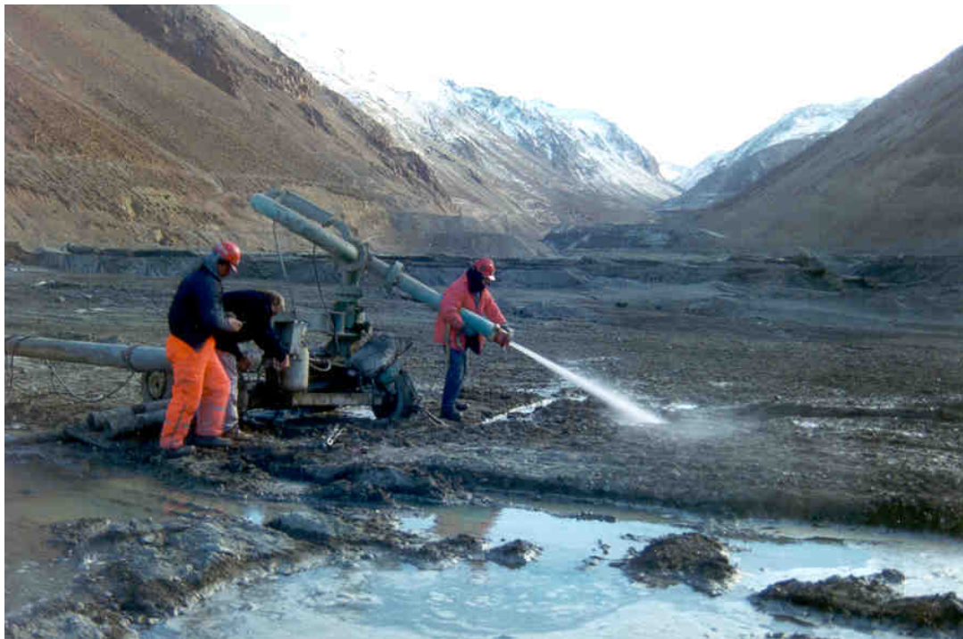
Photo 3.1a: A hydraulic monitoring gun in the Chilean Andes.
