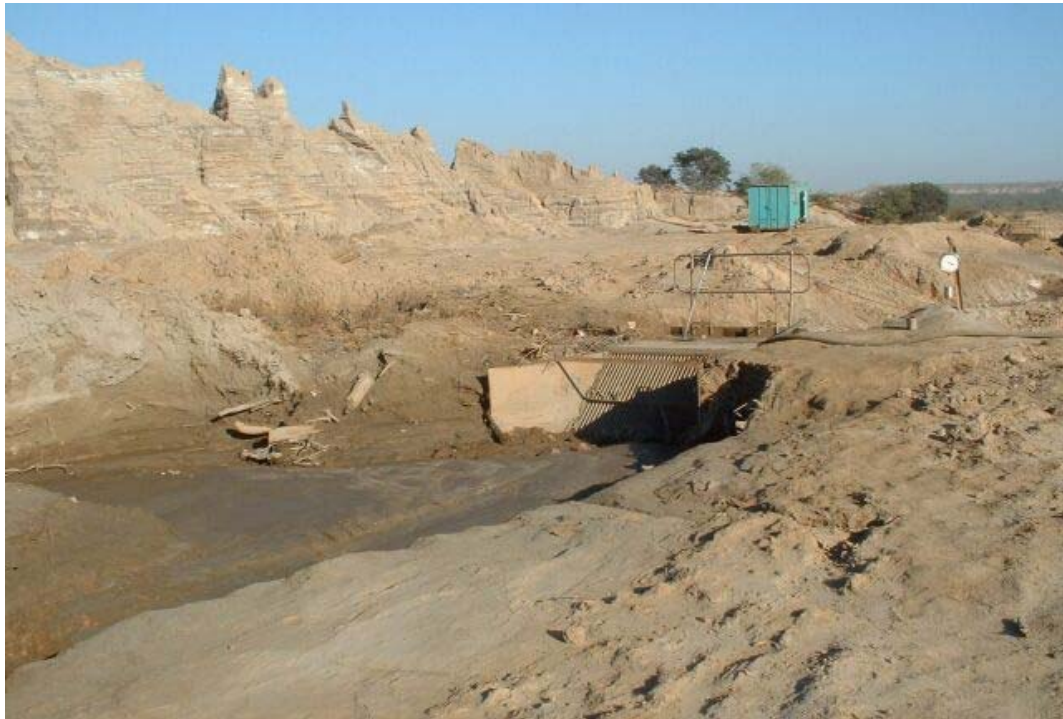
Photo 3.2b: Slurried tailings flowing through a grizzly prior to reporting to settling tanks and pumping station for subsequent deposition.
