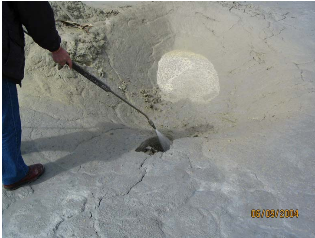
Photo 1.1B: Pressure washer was able to cut into the tailings surface adjacent to the Intermediate Dam with relative ease.
