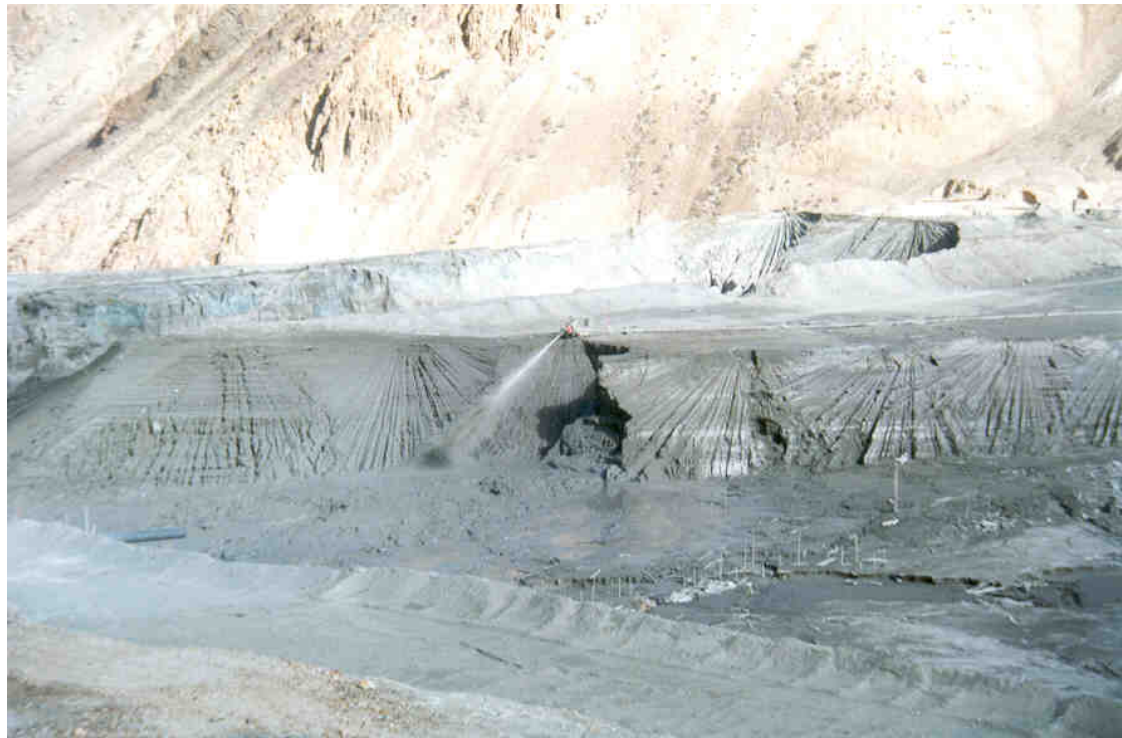
Photo 3.1b: Hydraulic monitoring from the top down.
