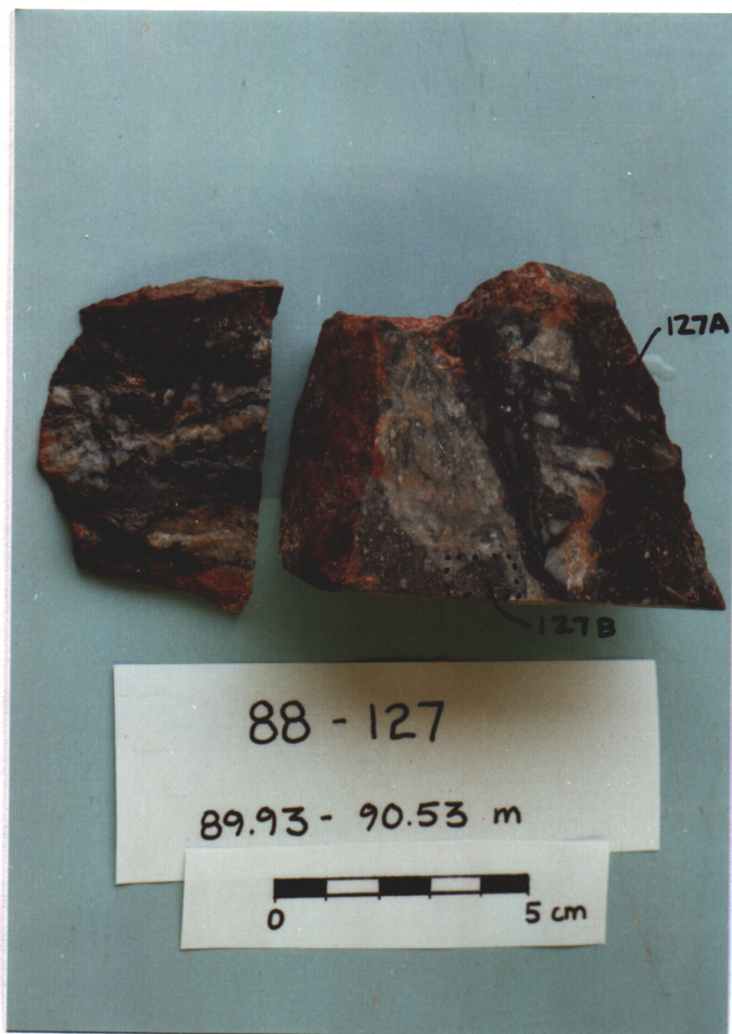
Photo 1 (left). Typical ore breccia, with silicified wallrock or vein fragments in grey-black matrix.
