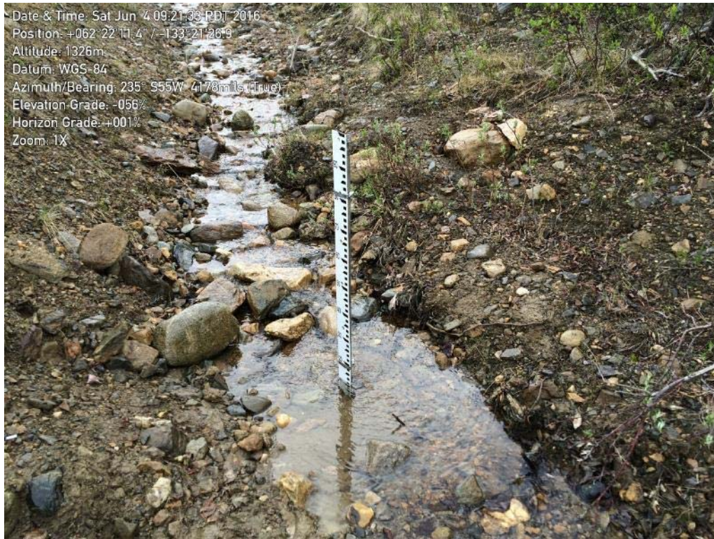
Photo 39. Streambed piezometer, installed with stage ruler, CH16-106-SG001
