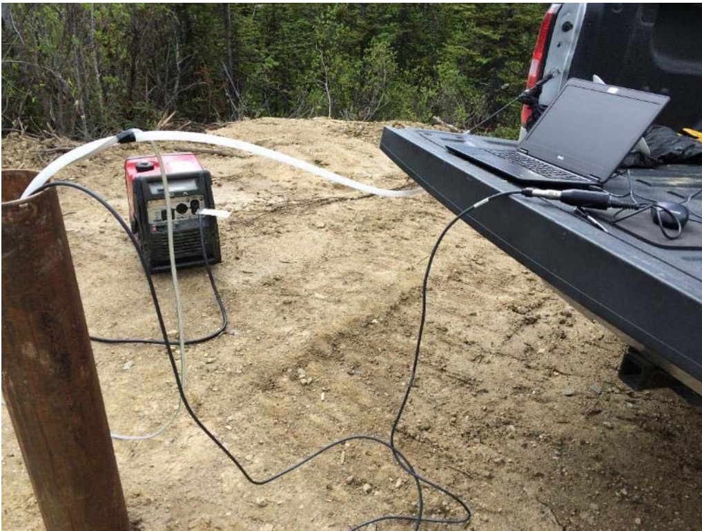
Photo 4. Computer connected to transducer cable; transducer deployed in CH15-106-MW007.
