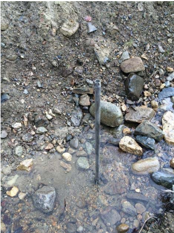
Photo 38. Streambed piezometer, installed
