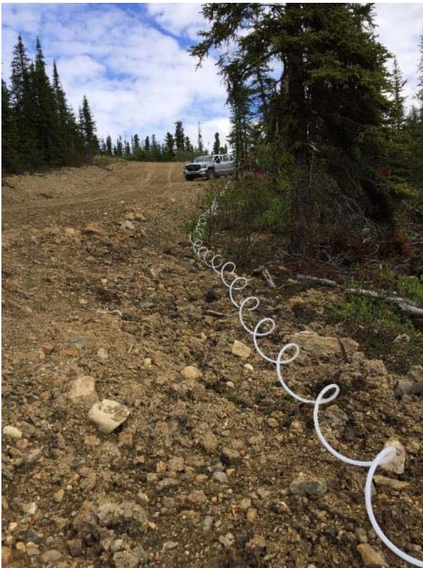
Photo 6. Discharge line running from CH15-106-MW007.
