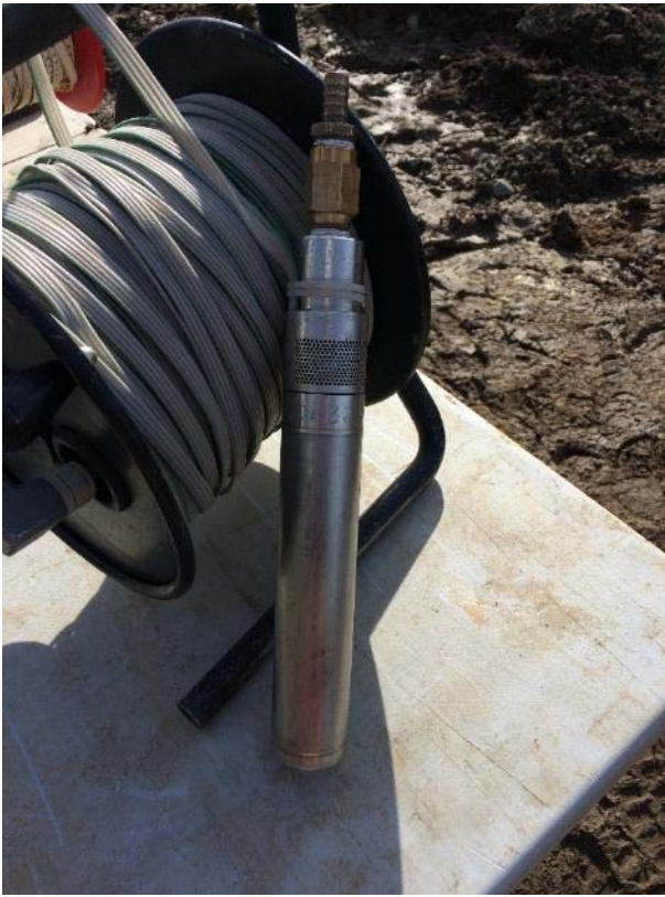
Photo 3. 2-inch Grunfos pump
