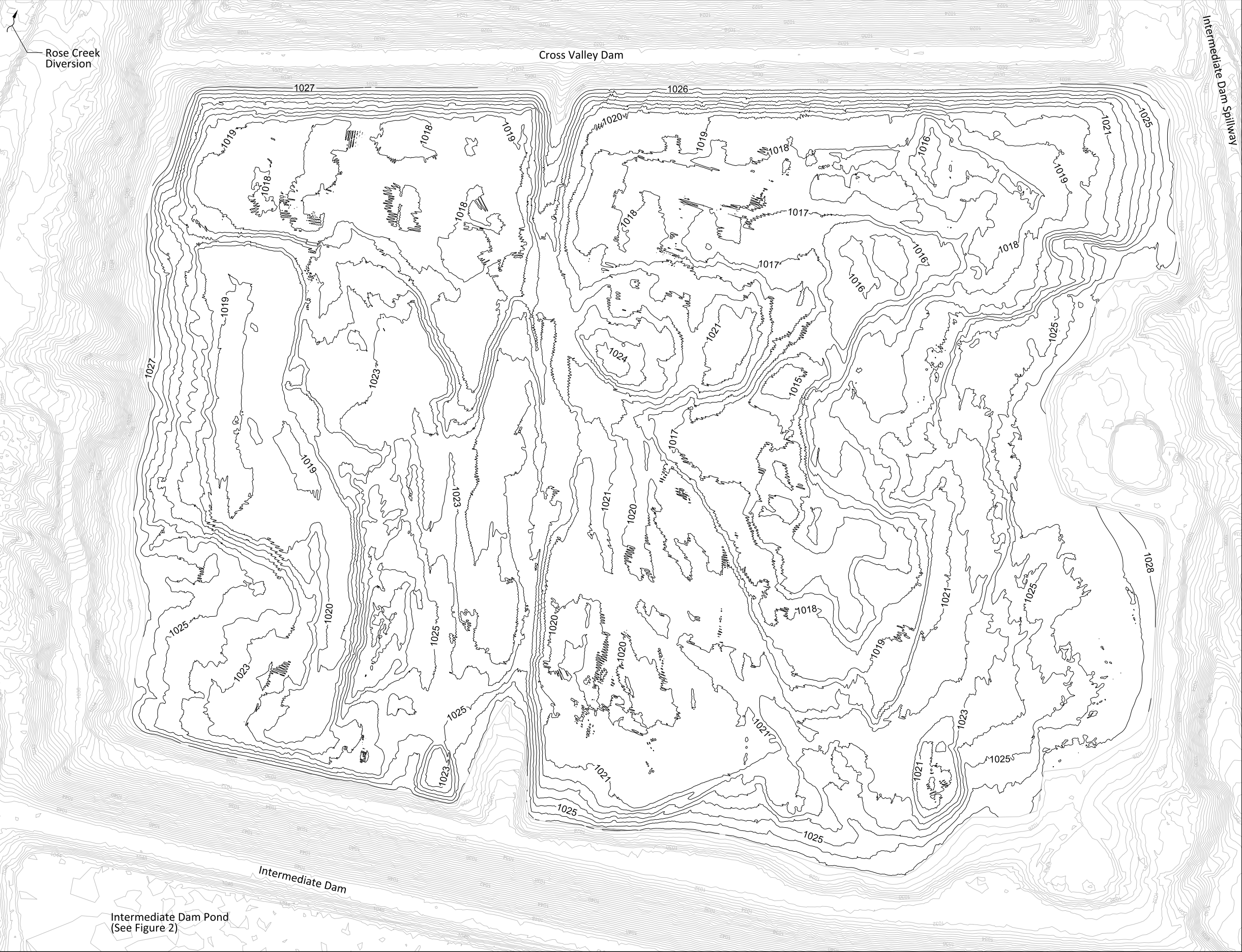
Figure 1 Cross Valley Pond Bathymetry Survey Faro mine Remediation Project Faro Mine Remediation Project
