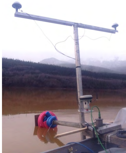
Figure 3: Universal mounting pole with three GPS antennae and subsea motion sensor visible.
