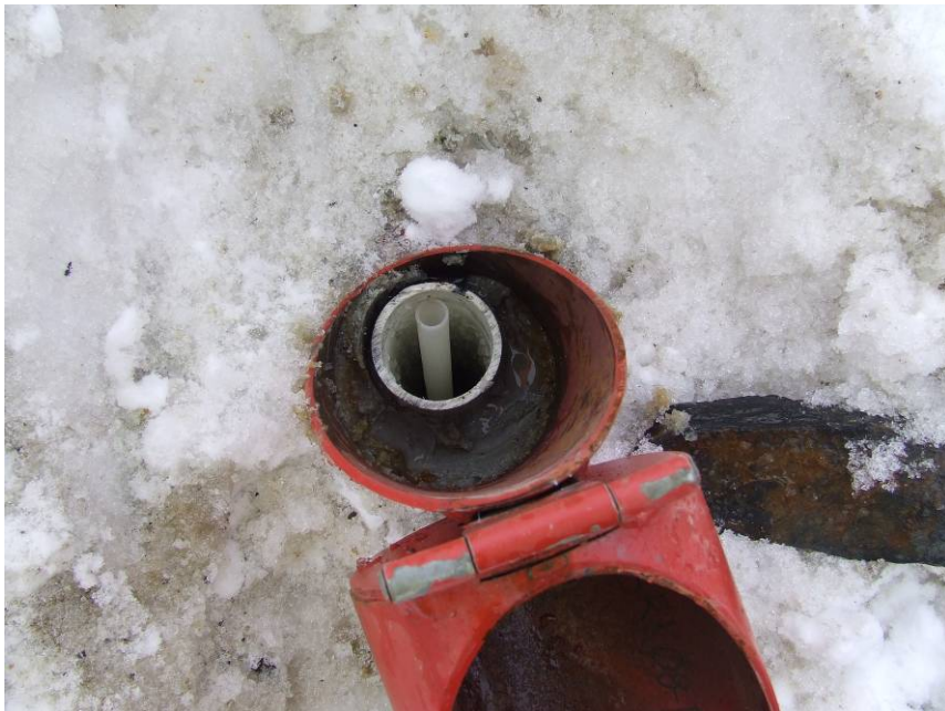
Well name: SRK08-P11A, drilling mud up to cap, May 15, 2012.
