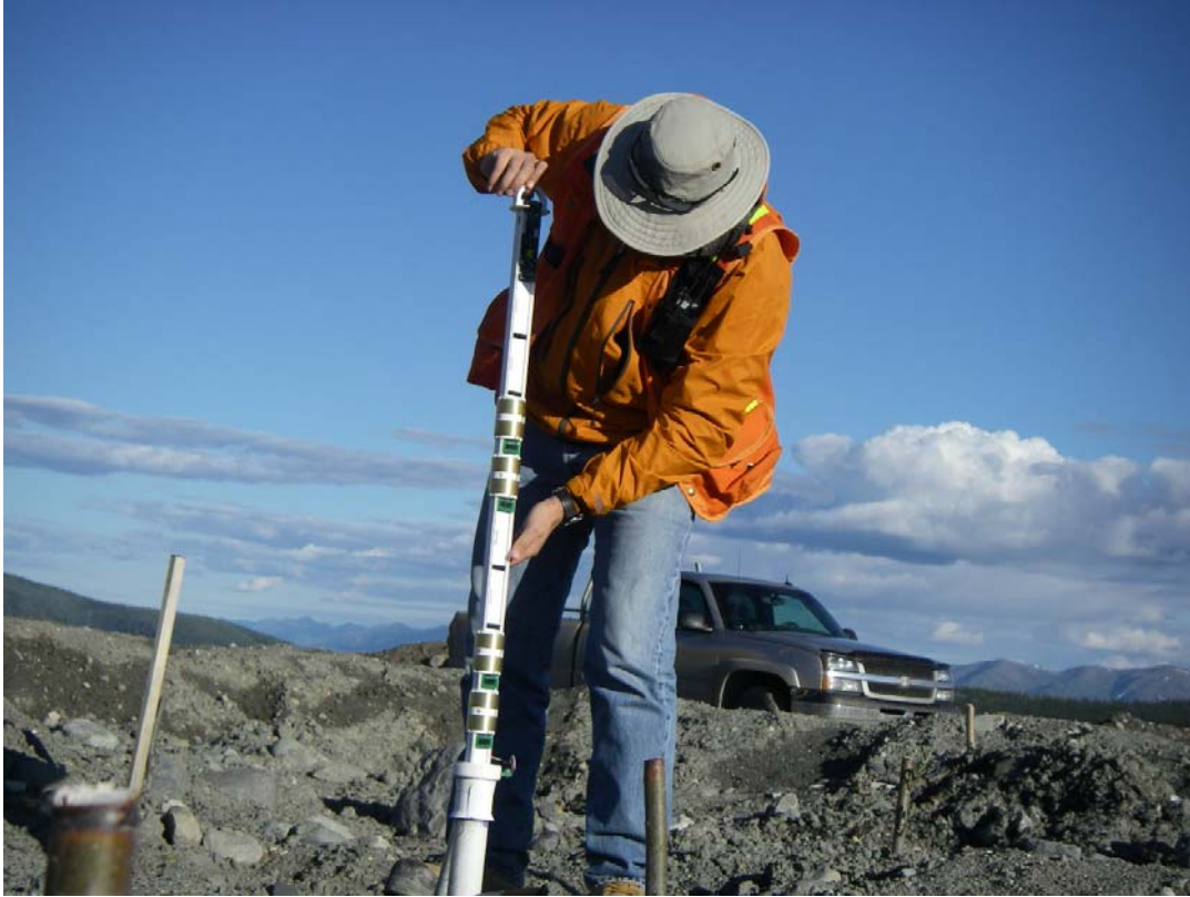
Photo 25: Sentek EnviroScan Probe Being Lowered Into Access Tube
