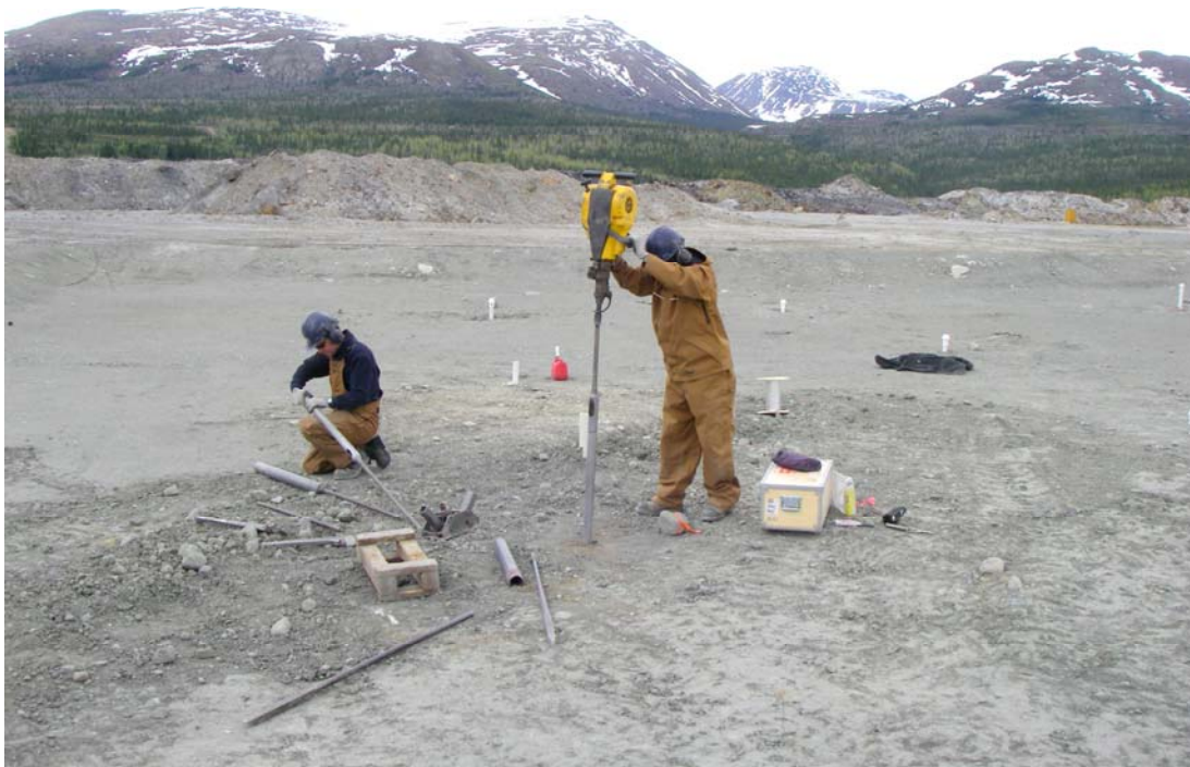
Photo 24: Drilling the Holes for the Diviner Access Tubes on L#2
