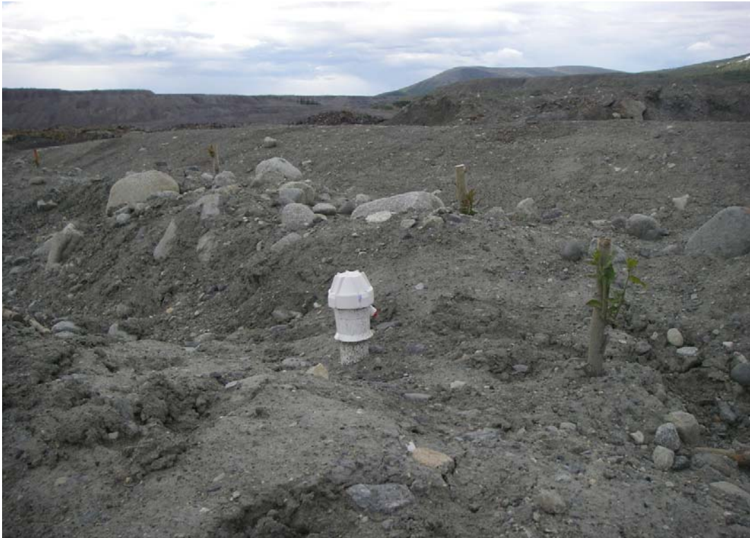
Photo 27: Top Cap Assembly of a Diviner Access Tube on L#1. Note that the cover was revegetated during fall of the previous year
