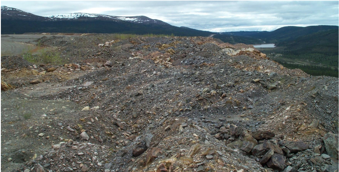
Photo 19: The waste rock can be anything from clay size particles to boulders.
