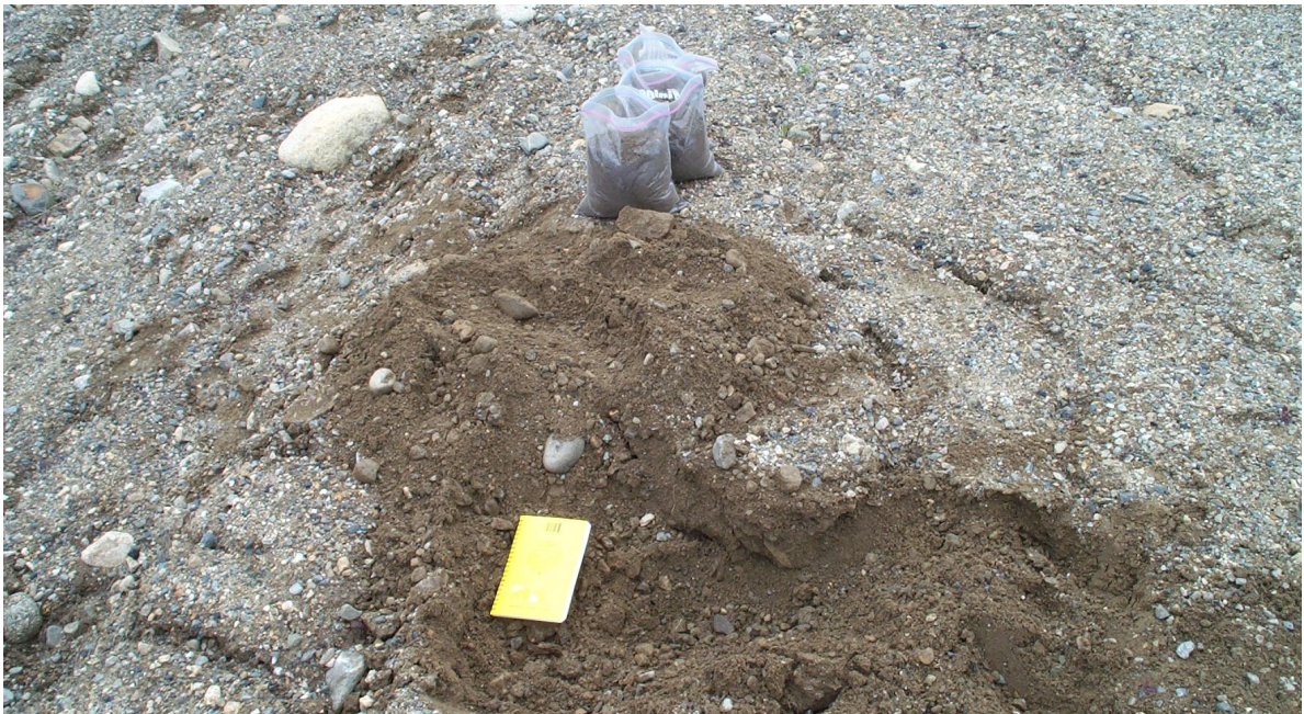
Photo 10: SRK-03-C03, glaciofluvial sample from north fork haul road borrow area. The sample excluded material that exceeded 50 mm (2") in size.
