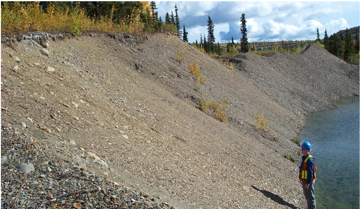
Photo 18: The second of two typical exposed glaciofluvial deposits. In these deposits, there are much less cobbles and boulders, and when present they are mixed throughout the matrix.
