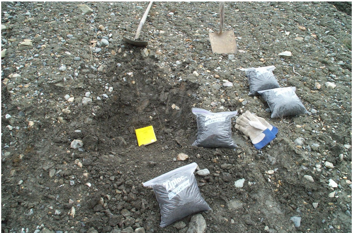
Photo 8: SRK-03-C01, till sample from the Vangorda waste rock pile cover. The sample excluded material that exceeded 50 mm (2”) in size.
