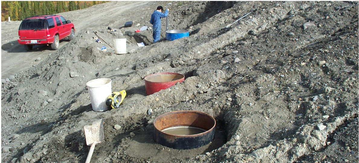
Photo 21: Sloped test site showing 3 ring infiltrometers being used for testing.
