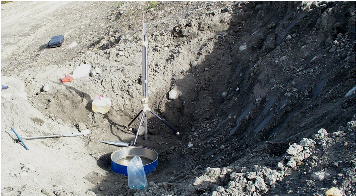
Photo 22: Test site showing a ring infiltrometer and Guelph permeameter.
