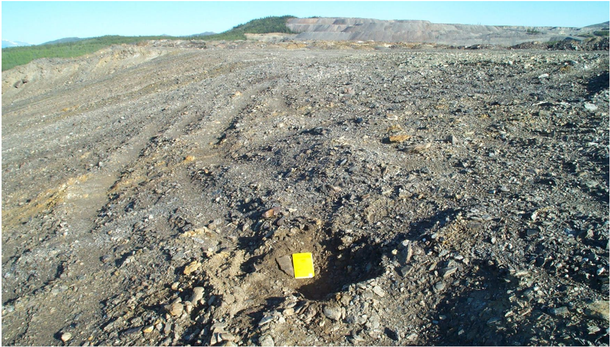
Photo 15: SRK-03-C08, re-handled waste rock from Vangorda waste rock pile. The sample excluded material that exceeded 50 mm (2") in size.
