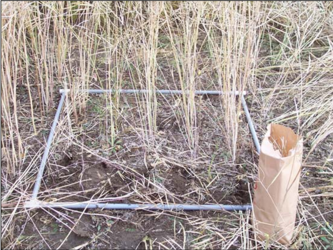
Photo 5: 1m 2 frame used to define the area to harvest
