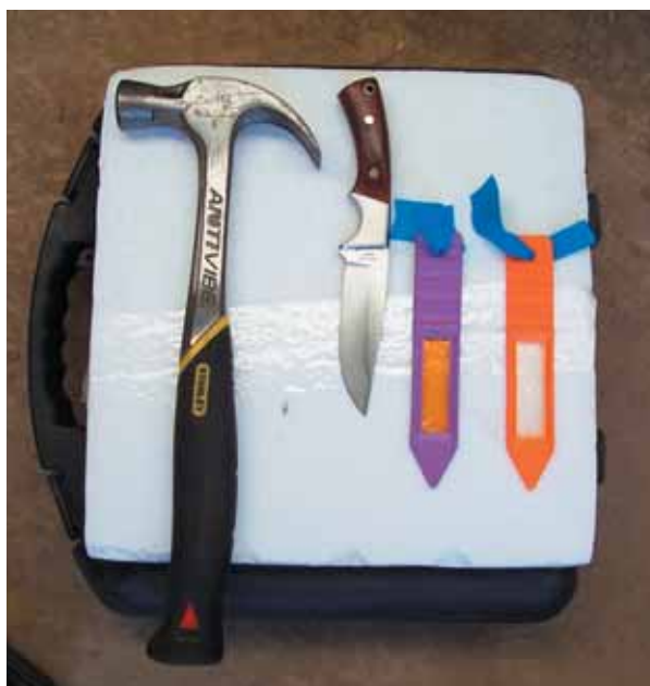
Photo 4.1 : Tools for PRS-Probe insertion, a knife to cut a slit, hammer to tap the probe into place, and the probes (purple - cation, orange - anion).
