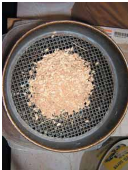
Photo 5.7 : Hand screens used to separate the seeds from a bulk of the scrap material left over from the thrashing.
