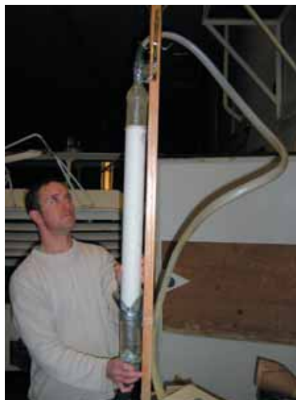
Photos 5.8 & 5.9 : A blower system set up to separate the finer scrap materials from the seed. Seed placed inside the tube on top of a fine screen and air was blown through the seed to push off any remaining scrap material.
