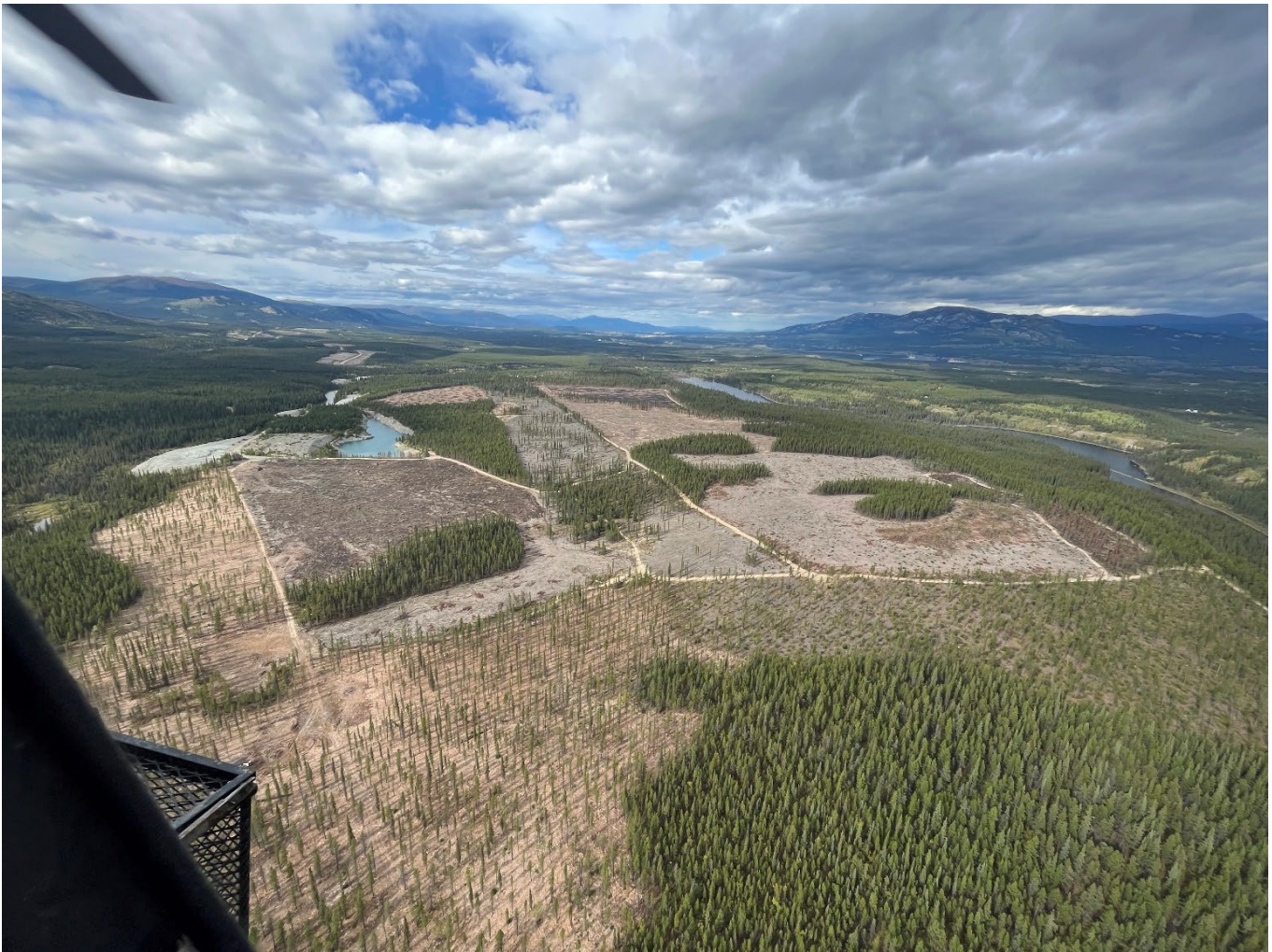
Figure 11: Example of the Mary Lake Shaded Fuel break in Whitehorse showing various fuel treatment techniques, including shelterwood thinning, variable retention (clearcuts), mastication (mulching) and prescribed burning.
