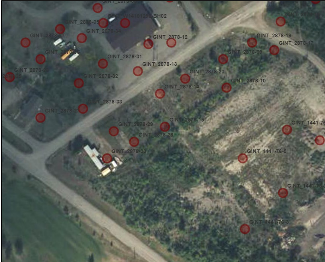
Figure B.3 – Geotechnical boreholes with drill records within the Study Area along Ladue Drive. The labels are the drill record number. There are 12 records within the planned lots; 8 of these had permafrost information. From Yukon Geological Survey, 2023.
