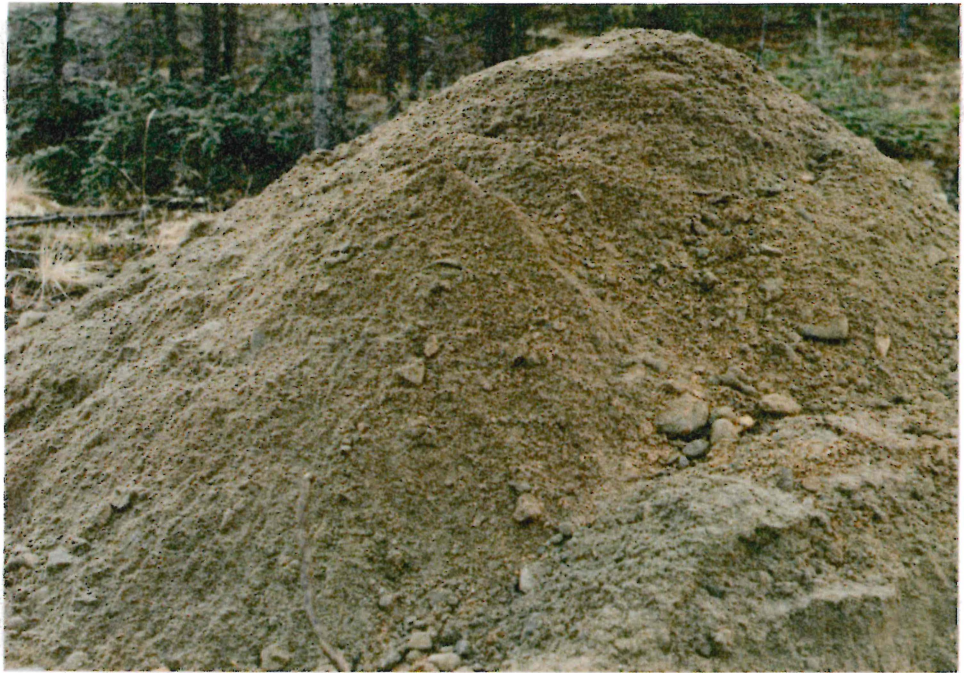
# 1-9 TP 86-3 EXCAVATED SOIL TO 1.7m DEPTH - SAND
