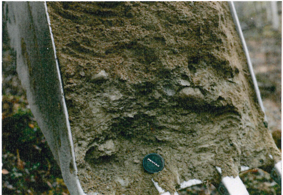
# 3-2 LAST BUCKET FROM TP 86-18 -BROWN SAND OVER GREY GLACIAL TILL
