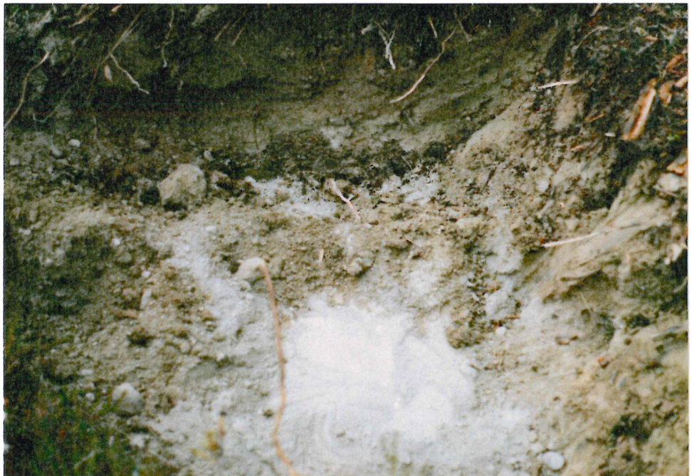
# 2-9 LOOKING DOWN TP 86-16 (ROCK AT BOTTOM OF PIT @ 0.4m)
