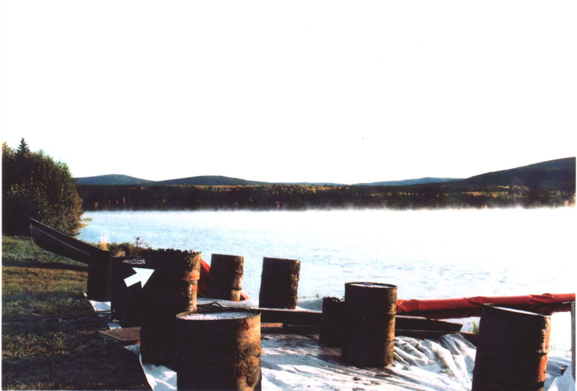
PHOTOGRAPH NO. 4: Recovered barrels at the Initial Attack Base. Note plastic ground sheet and half corroded barrel (arrow).
