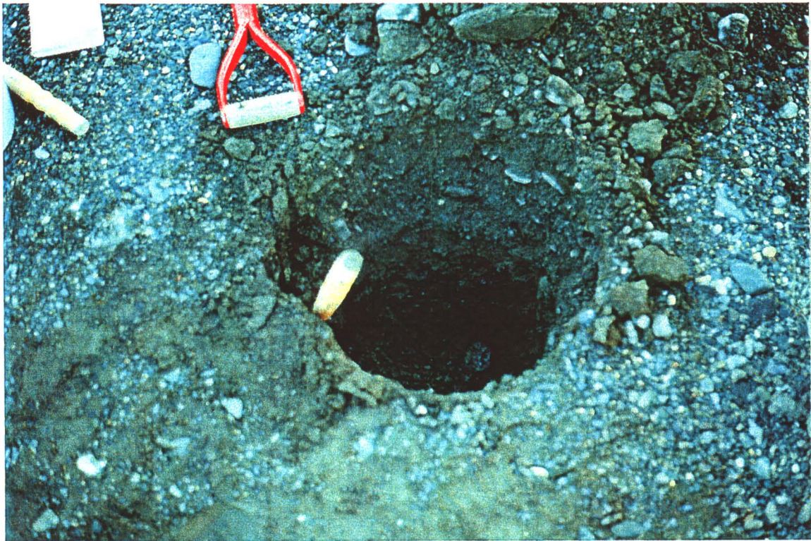
Photo 29: Granular material on the base of the bermed area surrounding the AST's.
