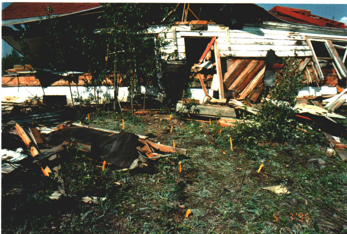
Photograph III-5: Delineation soil samples collected around G6100 which contained elevated concentrations of copper, lead and zinc.
