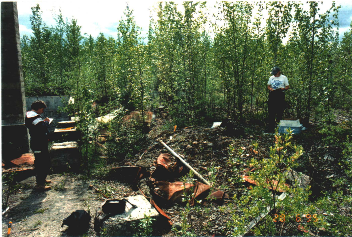
Photograph III-8: Samples collected off the west side of the barracks building foundation (G6116, G6117A/B) contained elevated levels of nickel, zinc and arsenic.
