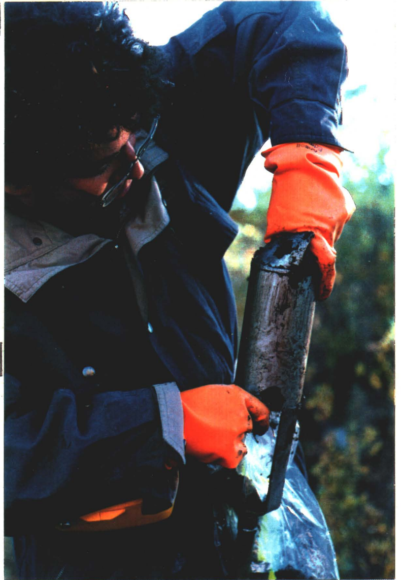
Photograph 30-P16: Removing portion of sample 30-S17 from auger.
