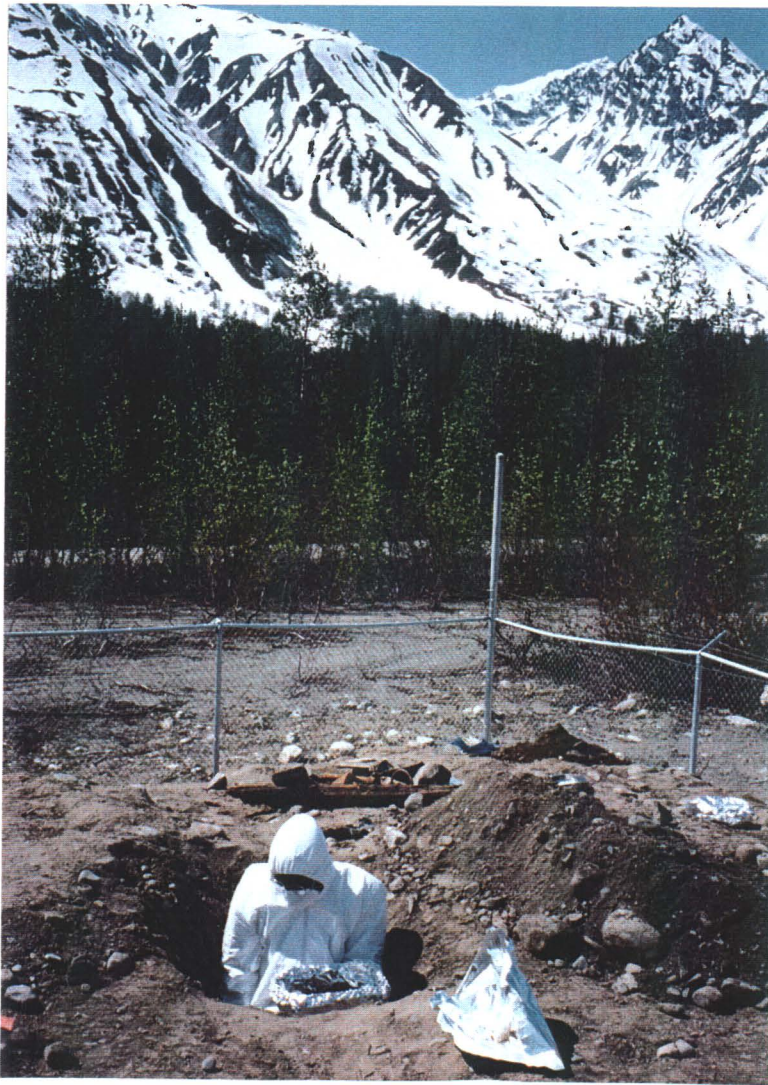
Photograph 2.5: Collecting a soil sample from a test pit at the Temporary Storage Facility
