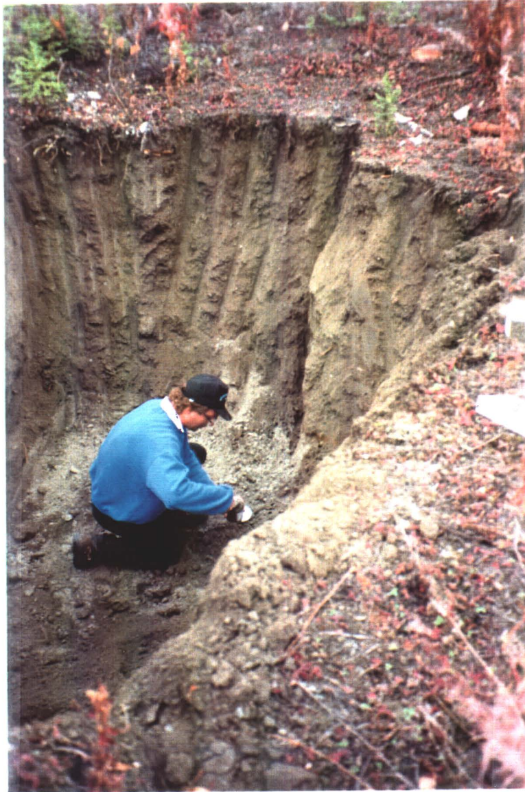
SITE 18 - Test pit, TP4, suspected location of underground storage tank
