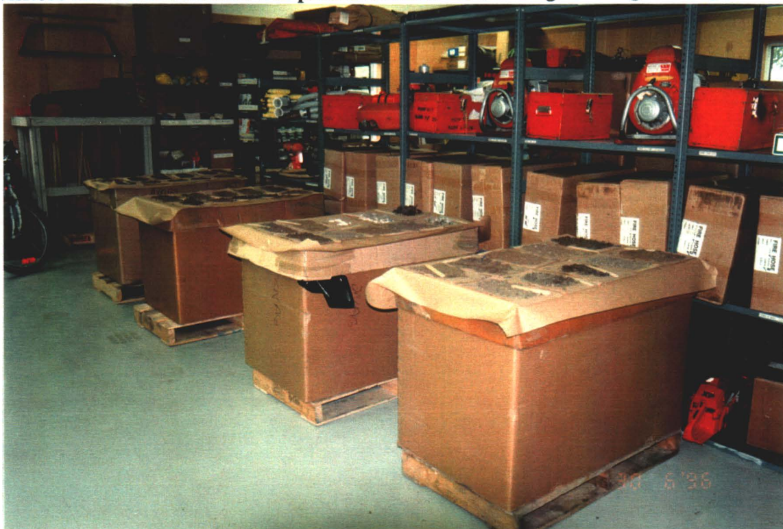
Photograph III-2: Soil samples were homogenized and laid out to dry on laboratory-grade paper towels before they were analyzed.
