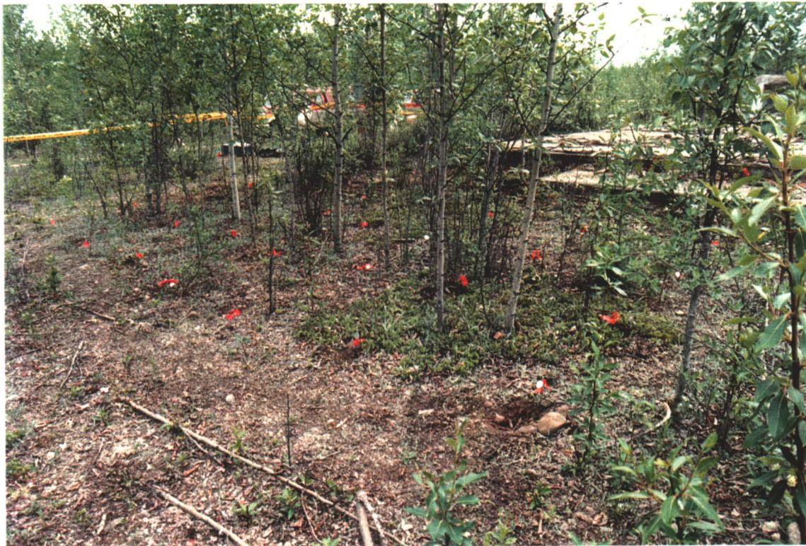
Photograph III-10: Delineation sample markers along the edge of the Powerhouse Foundation where soil was collected to determine the extent of PCB and metal contamination.
