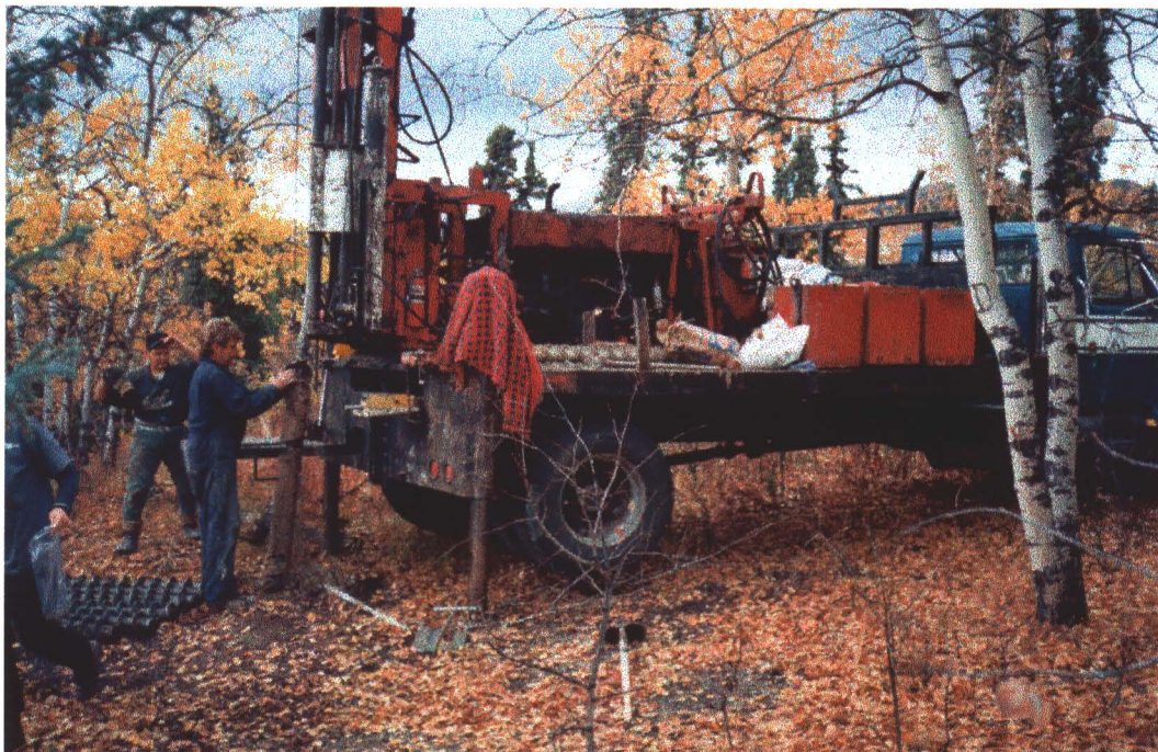
Photograph 18 - Mendenhall River - Truck mounted CME auger drilling rig used to install groundwater monitoring wells.
