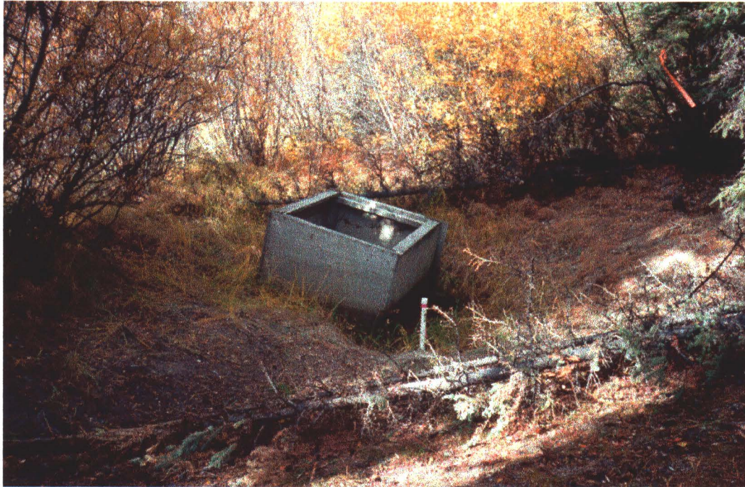
Photograph 21 - Mendenhall River - Typical monitoring well installed using small diameter hand auger.
