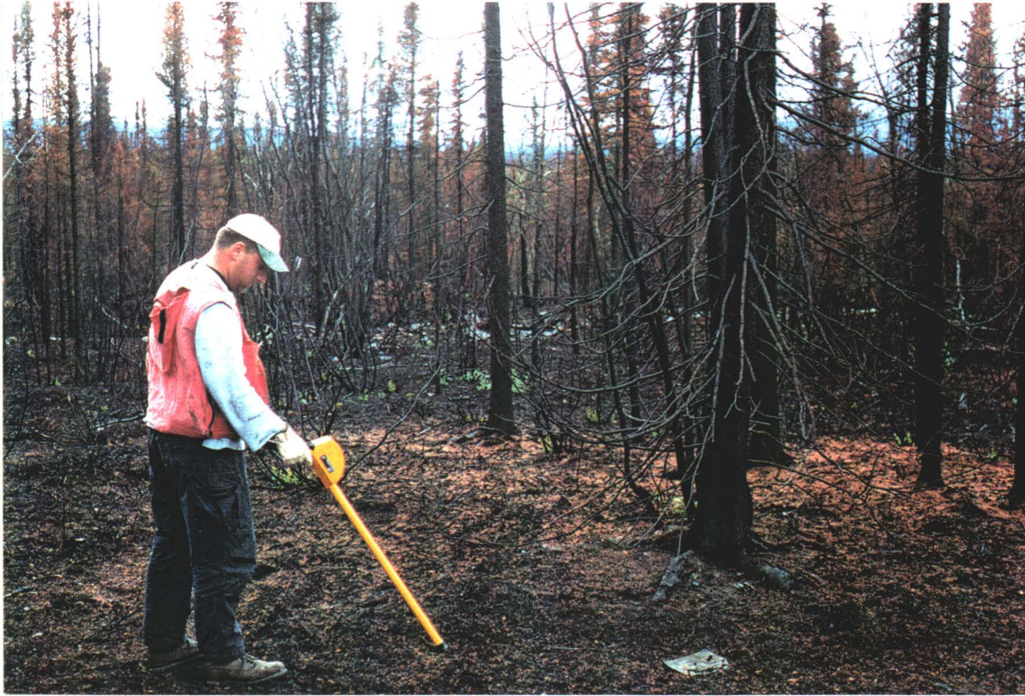
Searching for buried drums with metal detector.
