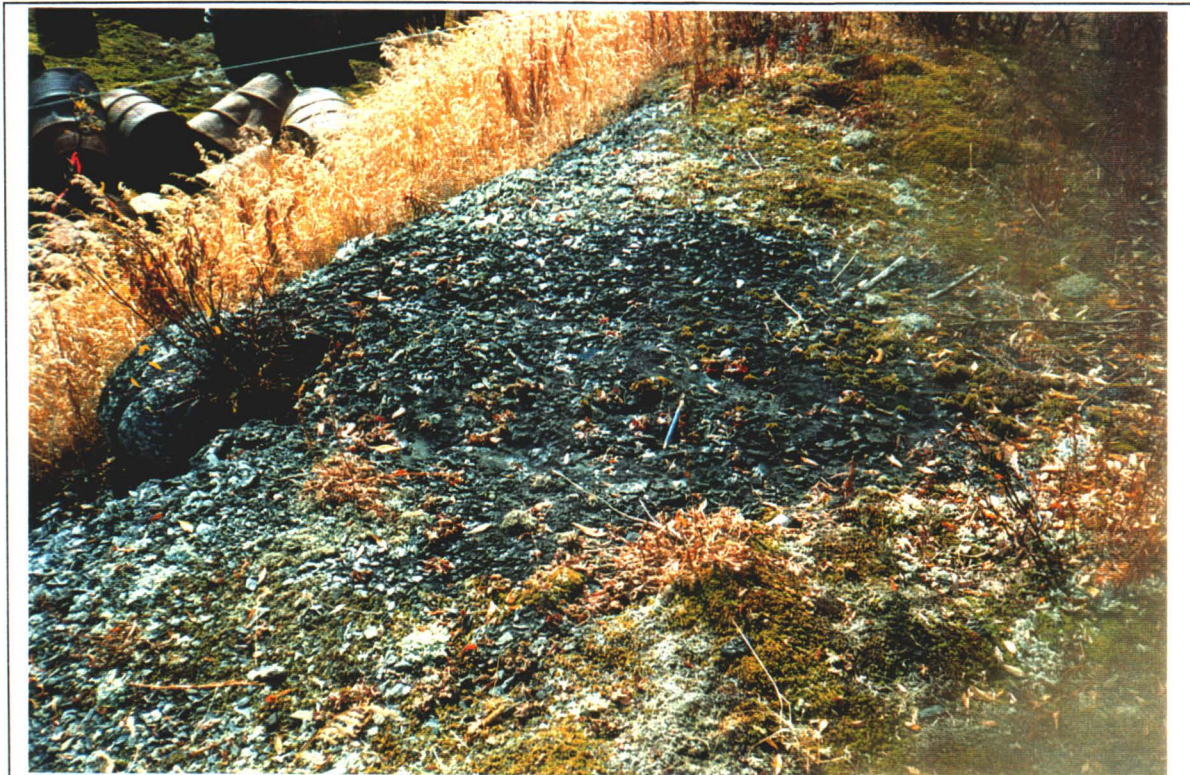
PHOTOGRAPH 25: Crude oil dried to asphalt like surface.
