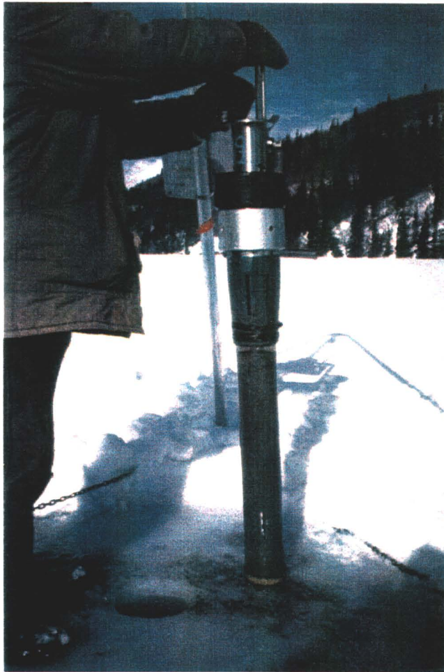
Figure 5: Sediment core from Klukshu Lake collected from deep portion of lake approximately in line with Gribble's Gulch
