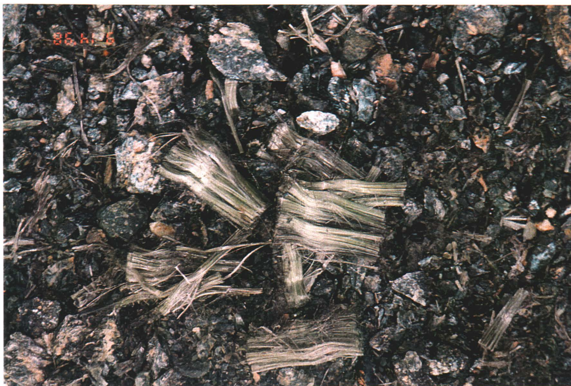
Photograph 2-5: Asbestos fibres amongst waste rocks at the Clinton Waste Rock Dump
