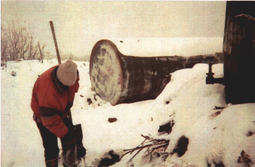
Photograph 28: Soil sampling at fuel tank # 1 showing berm and tank # 2 in background
