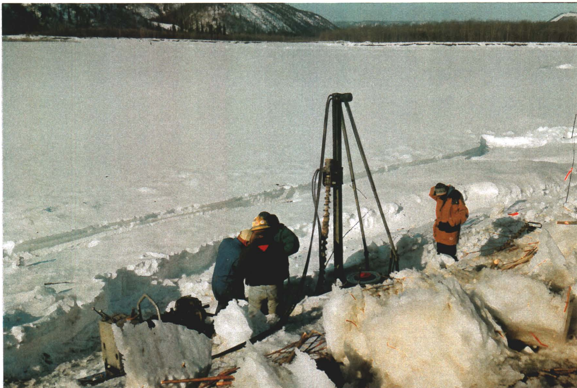
Photograph 2.4: Drilling with the solid stem auger along the cutbank
