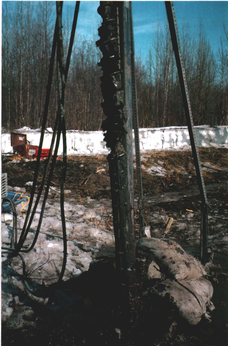
Photograph 2.5: Auger flight showing bentonite layer and other waste materials
