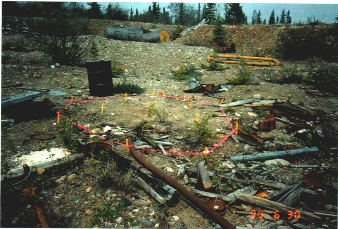
Photograph III-9: Delineation sample locations for east battery stain.
