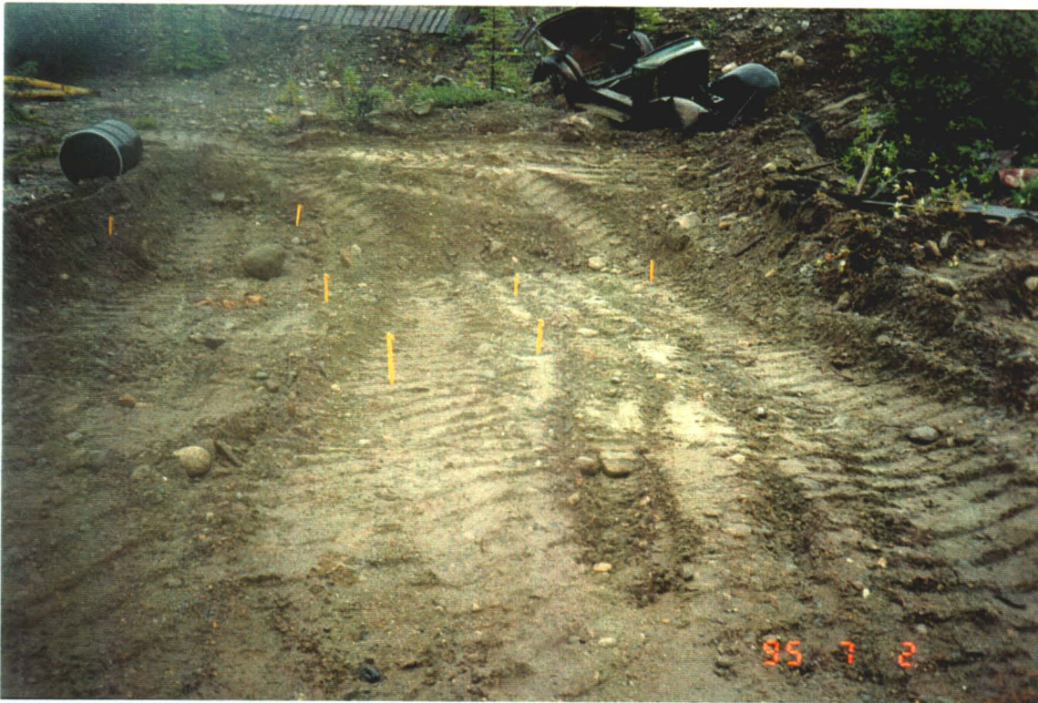
Photograph III-11: Confirmatory sampling at the east battery stain.
