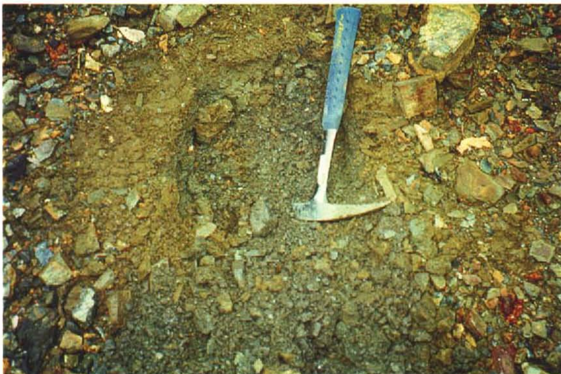
Photo 63-5: Test pit from waste rock pile #3. Note the oxidation at the surface of the pit. (Azimuth 240°)
