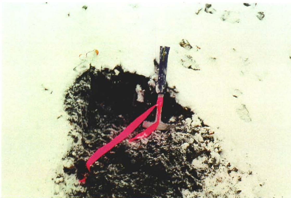
Photo 50-4: Test pit 1, waste rock pile #1. Note there is no oxidized horizon, only minor Fe-staining at the surface. (Azimuth 350°)
