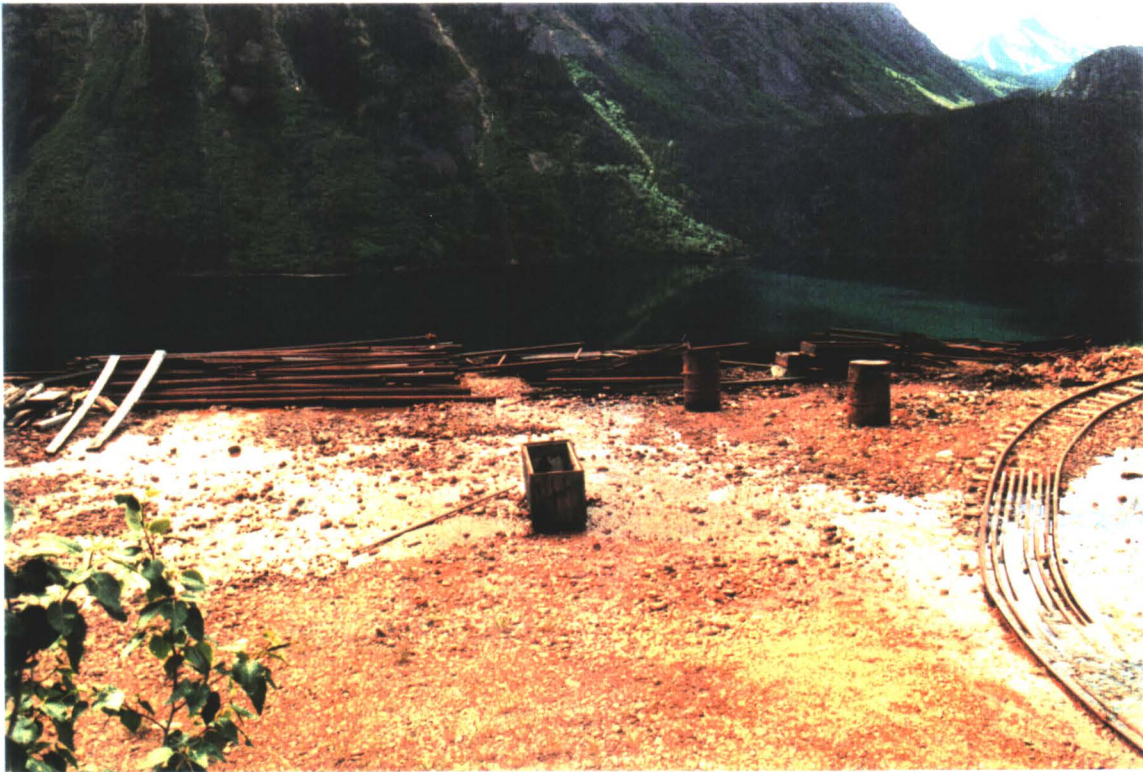
RAIL, BARRELS, AND PIPE ON WASTE PILE TO ADIT #1 (NOTE DRAINAGE)
