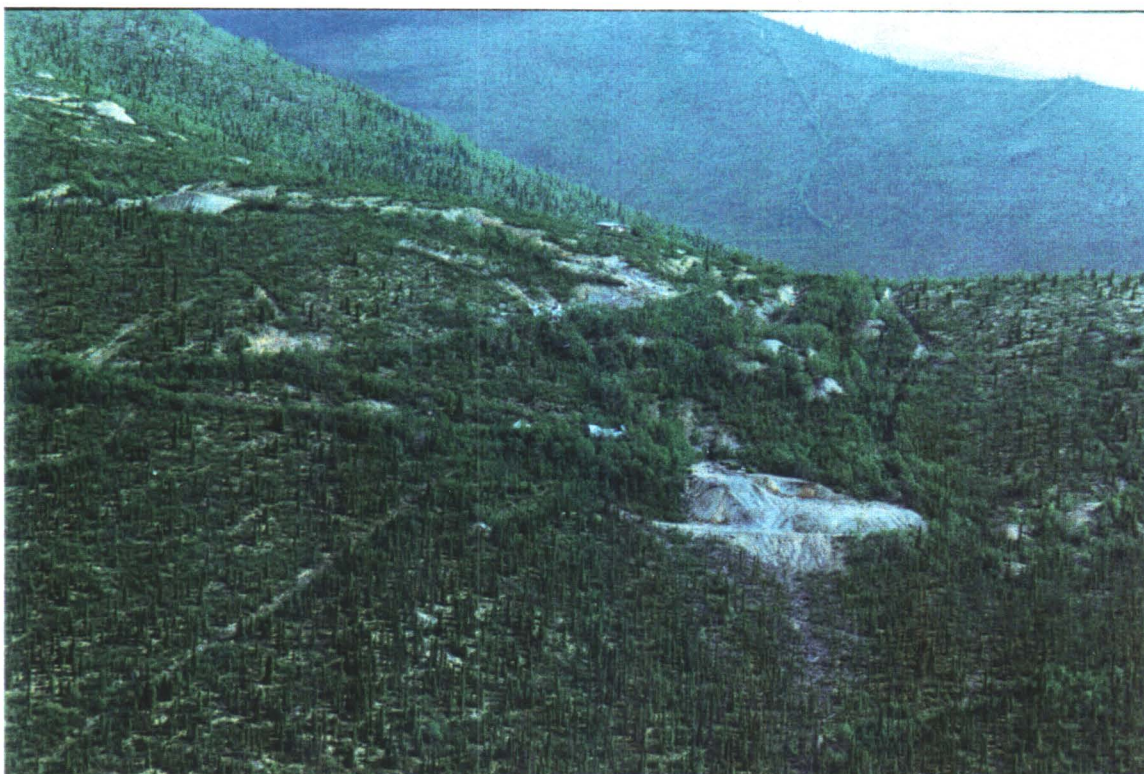
VIEW OF SITE. NOTE VEGETATION STRESS BELOW WASTE ROCK.
