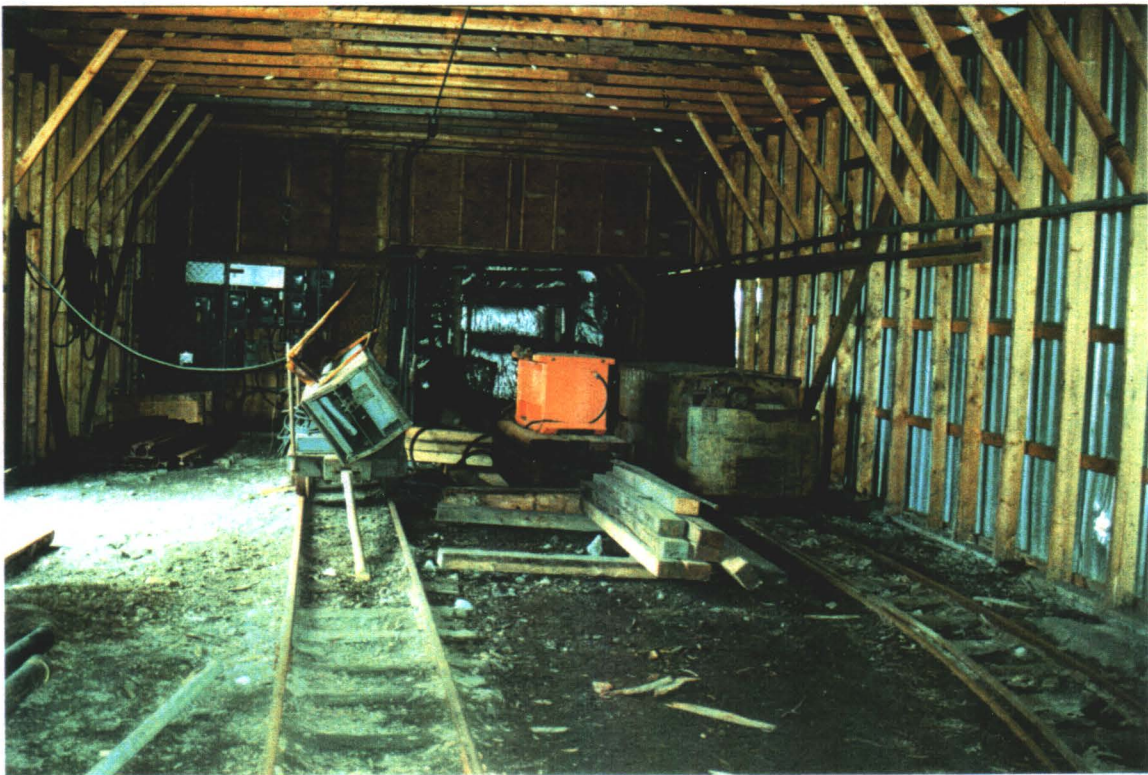
ENTRANCE TO ADIT, ELECTRICAL SWITCHING GEAR, AND LOCOMOTIVE INSIDE MINE ENTRANCE BUILDING
