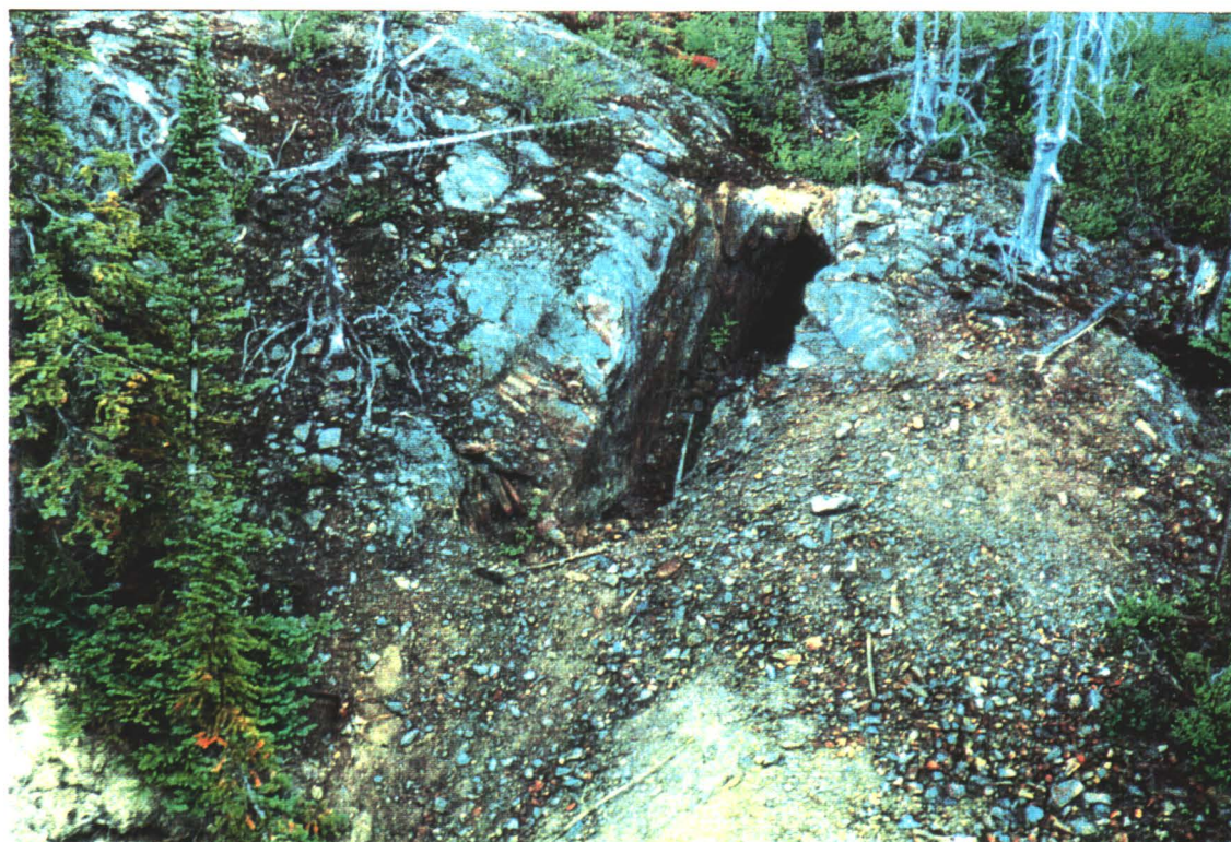
Photo 4: Adit and oxidized waste rock pile. Looking south. (Photo reproduced, with permission, from DIAND, 1994)
