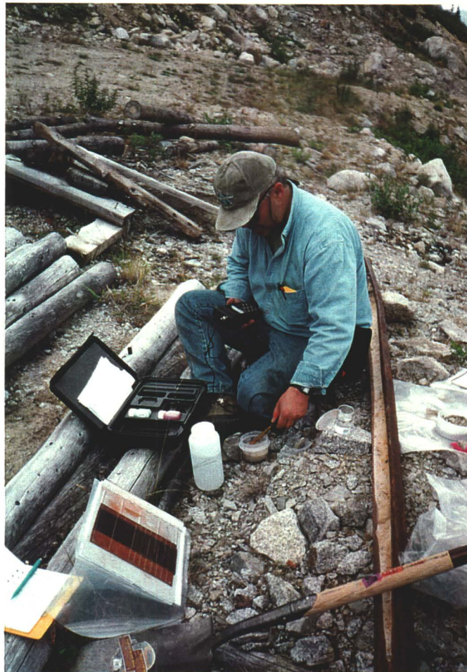
Photo 6. Determining conductivity during pH paste tests on waste rock samples at site.
