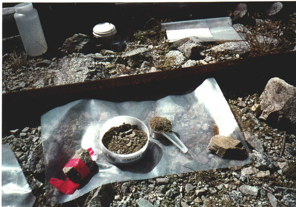
Photo 7. Preparing to place 65 ml sifted waste rock sample in beaker prior to determining paste pH and conductivity.
