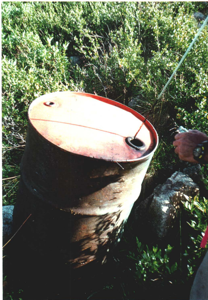
Photo 18. Use of 12 mm barrel drum thief to extract sample of petroleum hydrocarbon liquids for collection in sample bottles.
