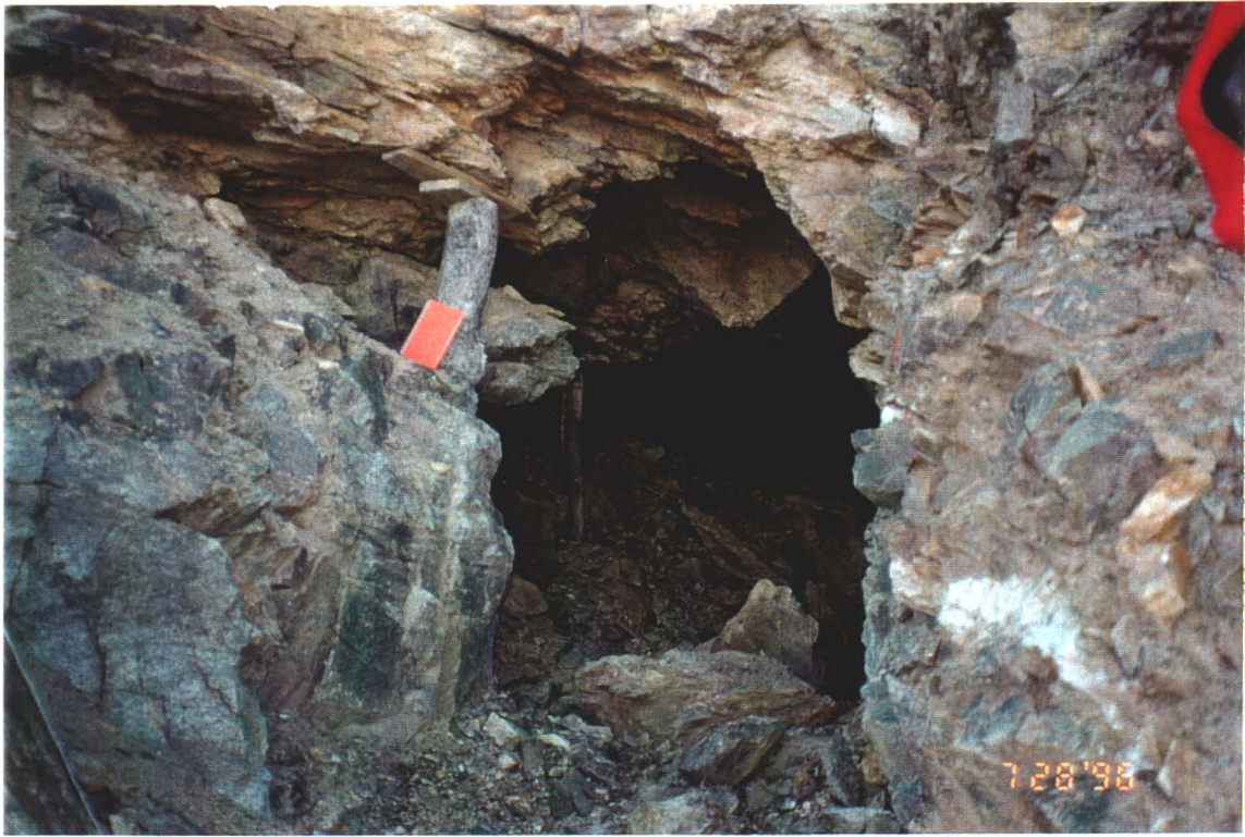
Photo # 1 - Open Adit in Side of Mountain
