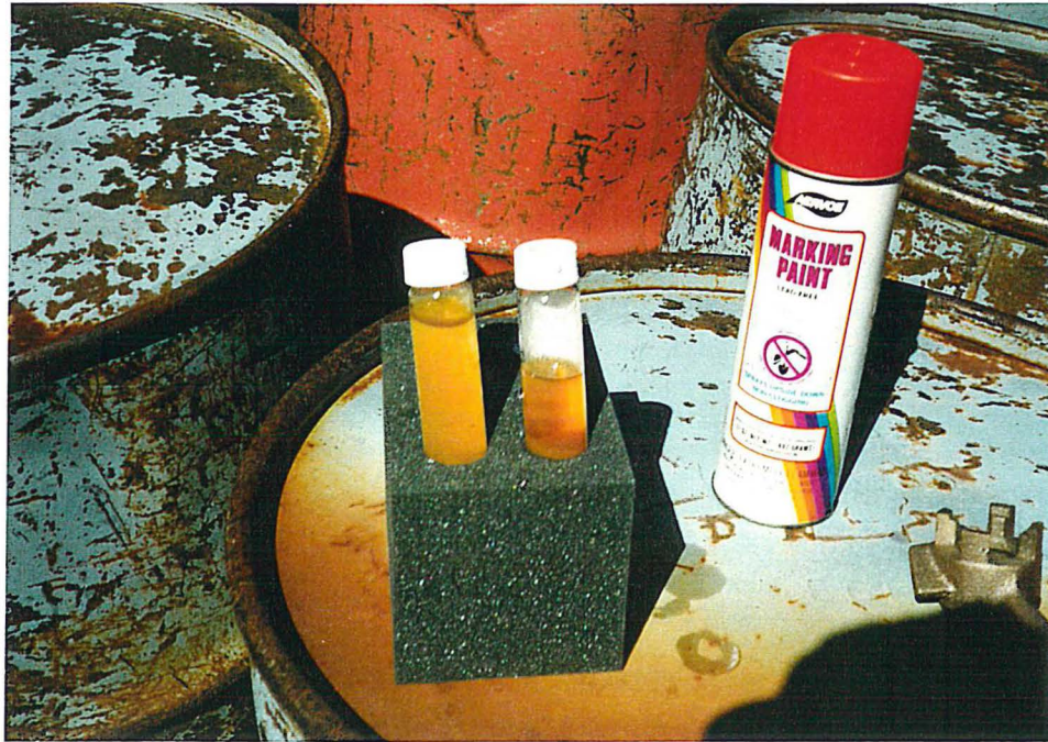
Photo 11. Purge and trap vials (40 ml) used during sampling of product of barrels.
